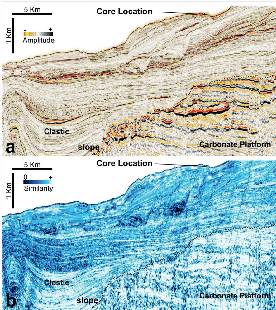
**Figure 4** Joint analysis of 3D seismic and core samples in the MSGBC Basin. This oil-bearing core is located over a fractured overburden along a regional migration pathway, connecting the Cretaceous carbonate platform with the clastic basin; a) Kirchhoff pre-stack depth migrated section; b) depth similarity attribute. Data was produced in partnership with TGS, PGS, GeoPartners.
