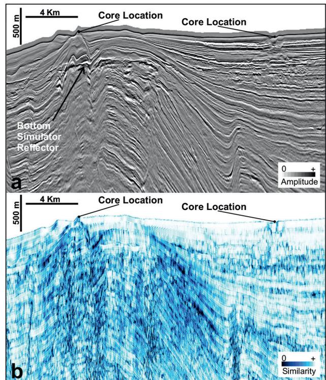
**Figure 6** Joint analysis of 2D seismic data and core samples in deepwater Nigeria. The cores are hydrocarbon-bearing, which are leaking to the seafloor from shallow fractures. Several stacked reservoirs are present in the subsurface fold, featuring a gas hydrate signature below seabed (bottom simulating reflector) a) Kirchhoff pre-stack depth migrated section; b) depth similarity attribute. Data was produced in partnership with TGS and Petrodata.
