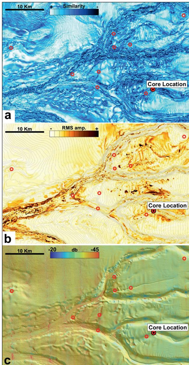
**Figure 3** Joint analysis between seismic and multibeam data in the MSGBC Basin. The 3D seismic attributes are extracted in the first 60 m underneath the seafloor. Water column anomalies are indicated as red circles; a) similarity, attribute (structural discontinuities); b) RMS amplitude attribute; c) multibeam bathymetry with backscatter overlay. Data was produced in partnership with TGS, PGS and Geopartners.
