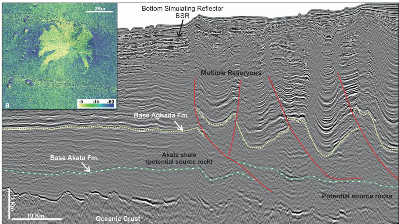
**Figure 5** The 2D Kirchhoff pre-stack depth-migrated section from deepwater Nigeria shows the main petroleum system elements. Inset figure a) shows the backscatter over a mud-volcano, the active seepage is visible of the bright flows on its flanks, presumably tars. Data was produced in partnership with TGS and Petrodata.
