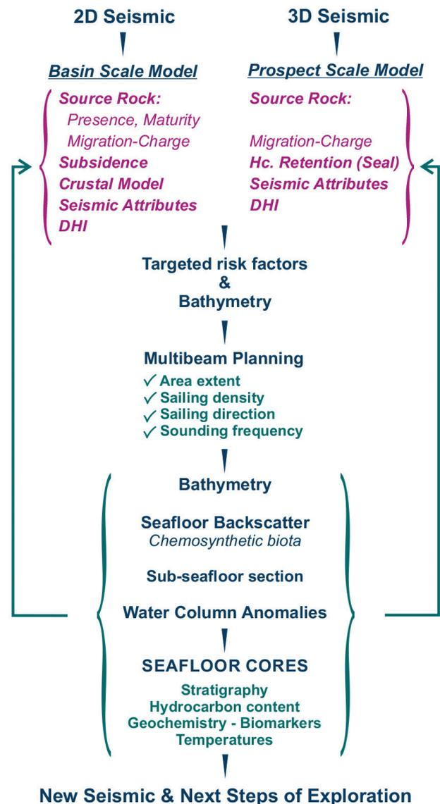
**Figure 1** Schematic workflow for integration of the multibeam and seafloor sampling in the seismic and exploration life cycle.
