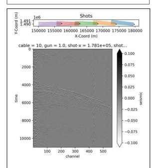
Figure 7: (Top): A Decimated streamer and shot geometry for a 3D offshore seismic dataset derived from MDIO coordinates. Bottom: A gather sliced from an MDIO dataset, showing gather for a specific cable shot, x/y combination.
