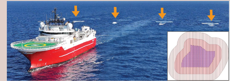
Figure 2: Amendment 4 acquisition: Gemini Source in quad-tow configuration and survey design showing the node placement, along with 10 km and 20 km shot halos.
