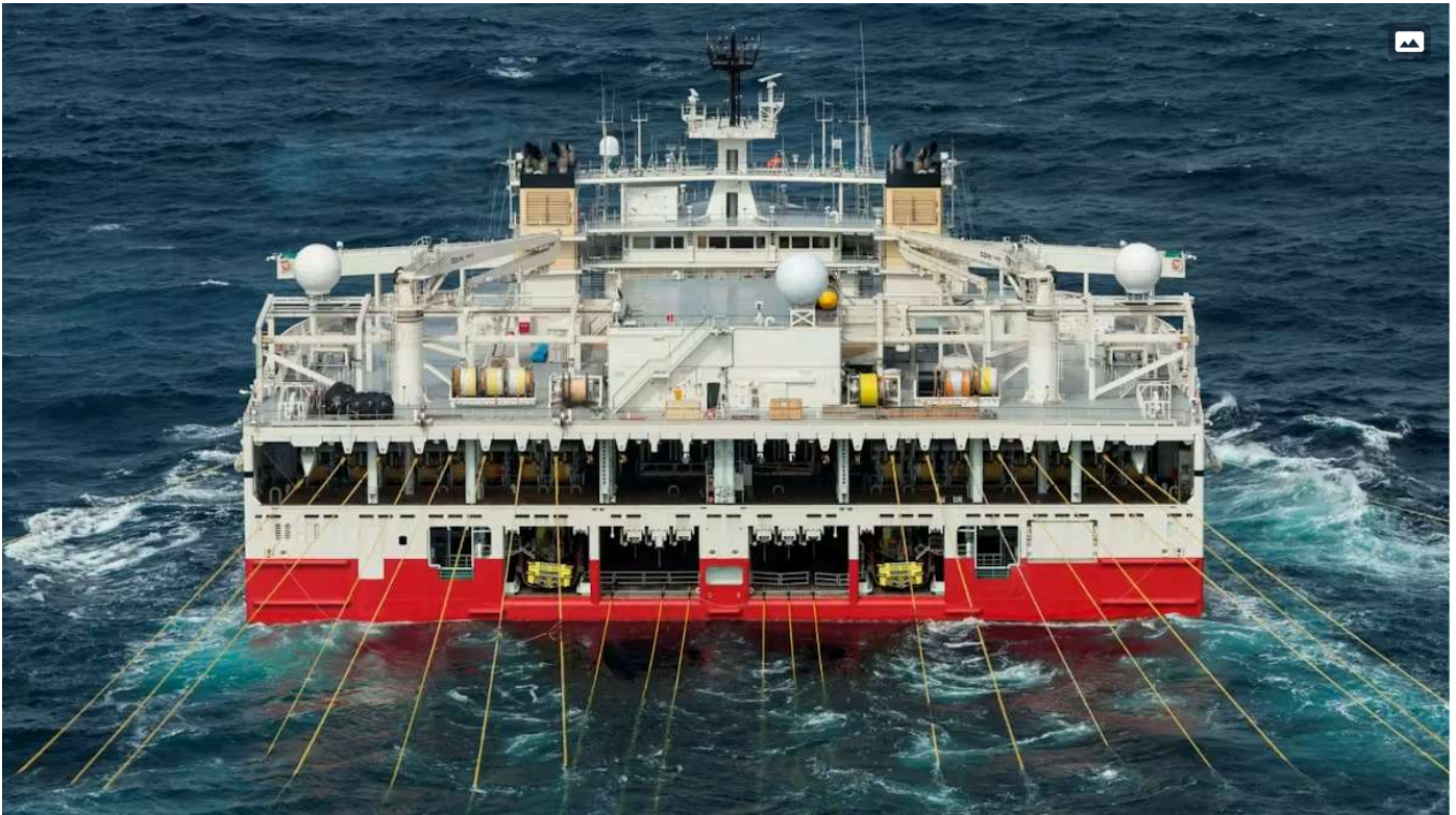
The Ramform Atlas vessel performs a towed streamer acquisition.
