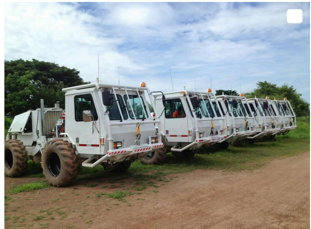
Seismic vibrator trucks perform land seismic surveys for oil and gas exploration in Thailand.
