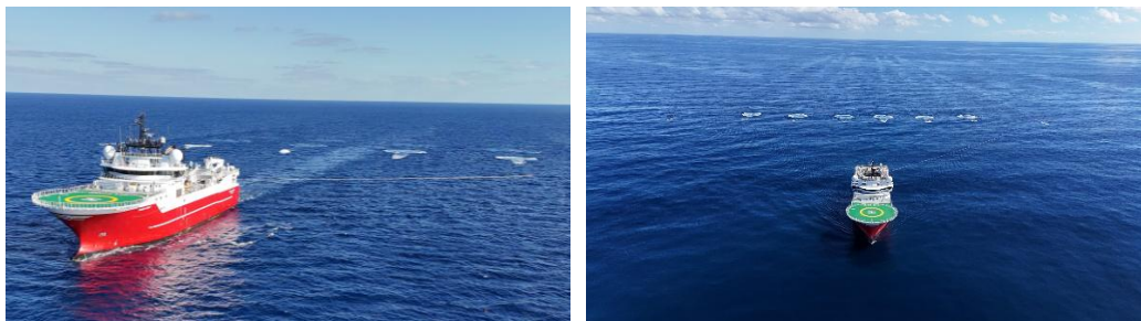
Figure 3 Acquiring data with extended-frequency source technology - efficient acquisition using wide-tow quad-source (Amendment Phase 4) and hexa-source subset (Amendment West 1).
