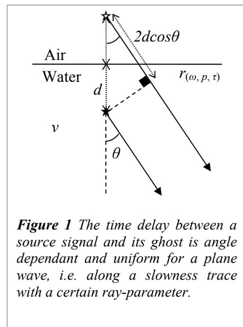
**Figure 1** The time delay between a source signal and its ghost is angle dependant and uniform for a plane wave, i.e. along a slowness trace with a certain ray-parameter.
