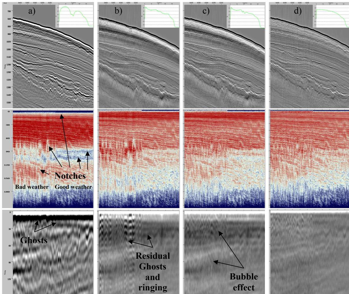
**Figure 3** A common- $p$  gather and its amplitude spectrum (top), the logarithmic amplitude spectrum and the autocorrelation of each  $p$ -trace (middle and bottom): a) before de-ghosting, b) after de-ghosting with nominal parameters, c) after de-ghosting with optimized parameters, d) after complementary deconvolution to remove remaining spectral defects including residual ghosts and bubble effect.
