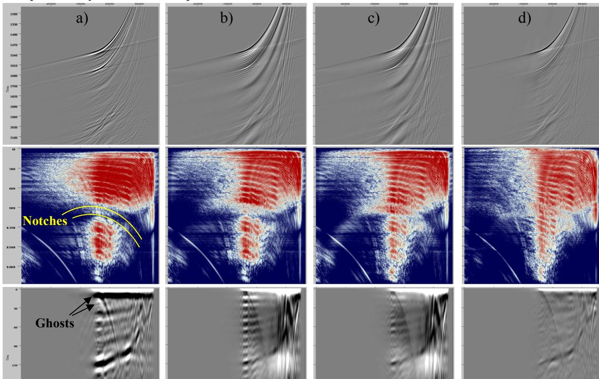
**Figure 2** A shot gather in the  $\tau$ - $p$  domain (top), the logarithmic amplitude spectrum and the autocorrelation of each  $p$ -trace (middle and bottom): a) before de-ghosting, b) after de-ghosting with nominal parameters, c) after de-ghosting with optimized parameters, d) after complementary deconvolution to remove remaining spectral defects including residual ghosts and bubble effect.
