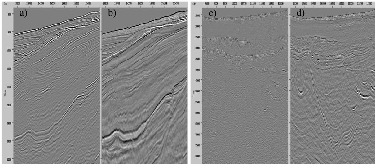
**Figure 4** A 2D profile from the West of Shetland basin with and without application of de-ghosting in the  $\tau$ - $p$  domain, deconvolution in common- $p$  and zero-phasing: a) and b) in a shallow zone, c) and d) in a deep zone. Note the improvement in resolution and also the enhancement achieved by exploiting the contribution from retrieved frequencies. Interpretable low-frequency signal is made available down to around 2 Hz.
