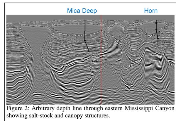
Figure 2: Arbitrary depth line through eastern Mississippi Canyon showing salt-stock and canopy structures.
