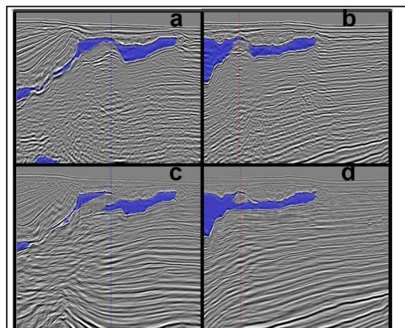
Figure 4: Shallow overhangs. (a) & (b) are orthogonal lines showing a simplified salt model. Note the image gap under the salt. (c) & (d) show the corresponding lines with the new interpretation. Salt shape is more complicated, but geologically simpler. The subsalt image is significantly improved.
