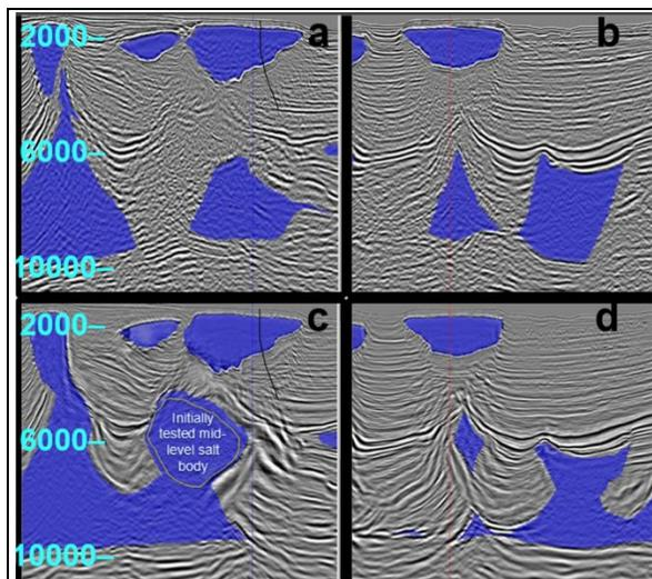
Figure 7: (a) & (b) are orthogonal lines with an earlier interpretation and resulting image. (c) & (d) show the corresponding lines with the new interpretation and improved imaging of the deeper section. Critical to the new interpretation is the addition of the mid-level salt body, labeled in (c).
