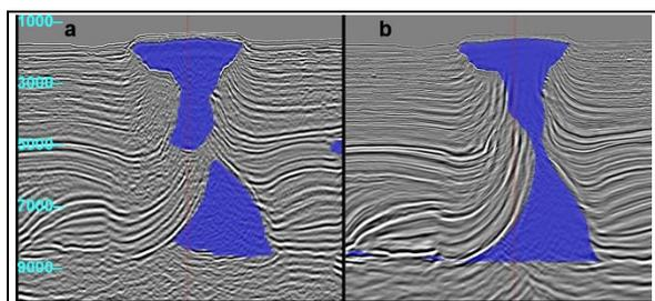
Figure 5: (a) Earlier model with early Miocene canopy included interpretation at 5200m. (b) Removing the canopy simplifies the model and helps in imaging of a megaflap along the salt flank.
