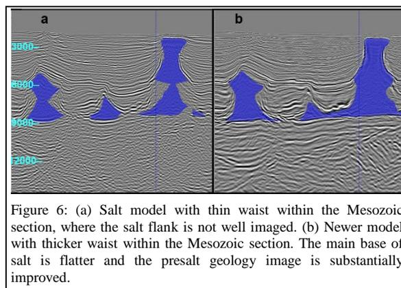
Figure 6: (a) Salt model with thin waist within the Mesozoic section, where the salt flank is not well imaged. (b) Newer model with thicker waist within the Mesozoic section. The main base of salt is flatter and the presalt geology image is substantially improved.
