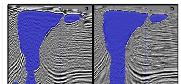
Figure 3: Subsalt illumination improvements. (a) WAZ image. (b) Long offset M-WAZ image with similar model
