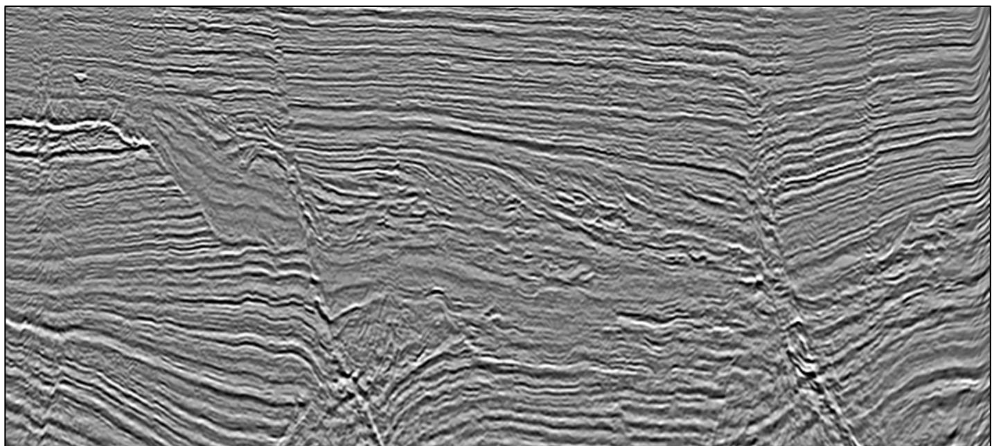
MegaSurvey 3D example from the vicinity of PPL 2A39. Structural, stratigraphic and combination traps are present.
