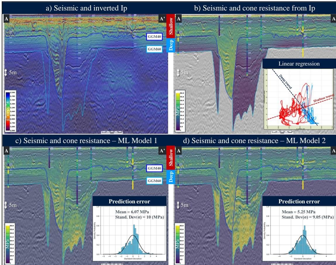
**Figure 3** (a) absolute acoustic impedance; (b) predicted cone resistance from the linear regression; (c) cone resistance prediction using ML Model 1; (d) cone resistance prediction using ML Model 2. The linear regression method does not manage to capture varying trends within the tunnel valley (deep interval), and there is not enough statistically meaningful information for splitting the deep window into another interval. Breaks in trends are well-handled by both ML models.
