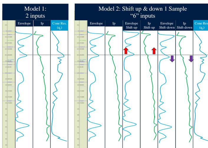
**Figure 2** Summary of two ML training datasets used in the study. By shifting upwards and downwards one sample envelope and inverted Ip it's possible to increase the number of inputs to train the model while proving the model a potential way for compensating for time-depth scaling mismatches.
