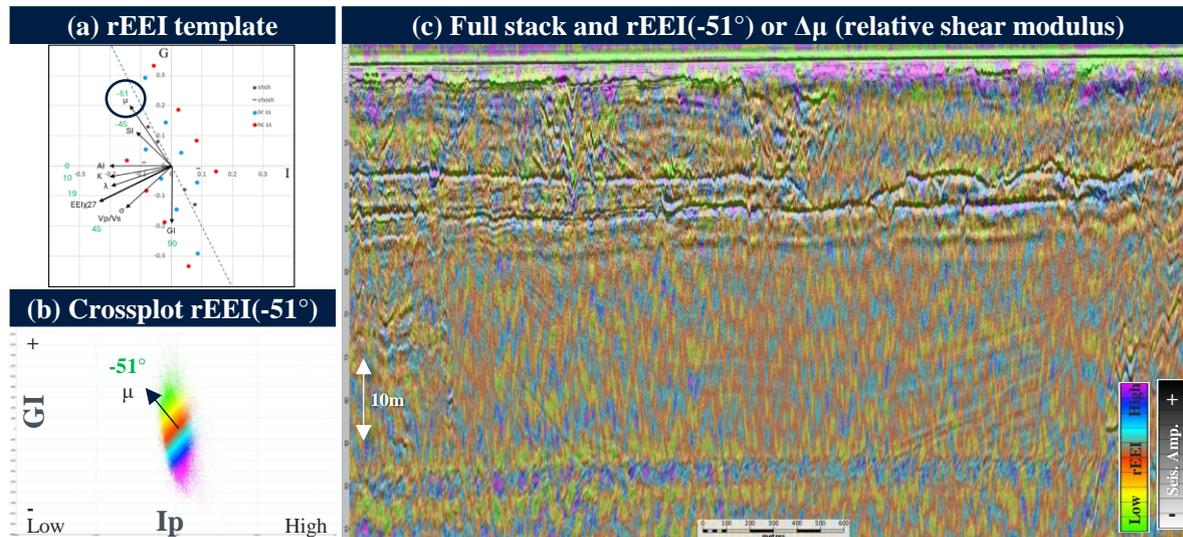
**Figure 4** (a) template showing the rotation angle to generate different elastic properties. The angle to estimate  $\Delta\mu$  (relative change in shear modulus or  $G_{max}$ ) corresponds to  $rEEI\chi = -51^\circ$  based on a generalized rock physics model (after Went 2025); (b) AI-GI cross plot coloured by  $rEEI\chi_{-51}$  (relative change in  $\mu$  or  $G_{max}$ ); (c) stack reflectivity co-rendered with inverted  $rEEI\chi_{-51}$  (relative  $G_{max}$ ).
