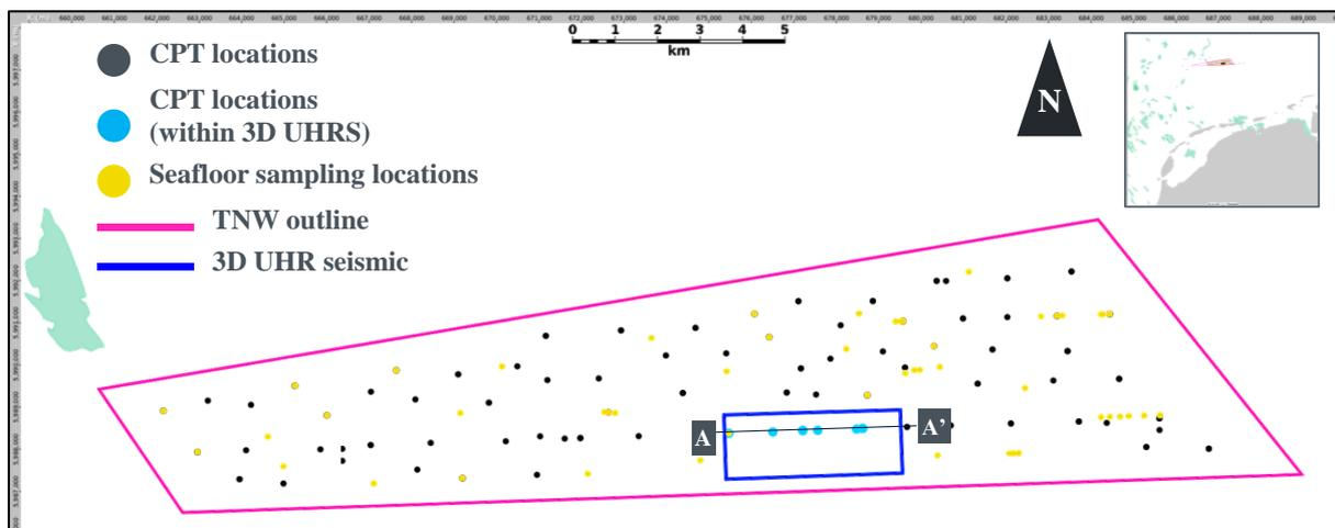
**Figure 1** Basemap showing outline of the TNW site and outline of the 3D UHRS data available for this study. Black dots represent CPT locations and yellow dots seafloor samplings. CPT locations used for training the ML model are in light blue. Prediction results are presented along profile A-A’.
