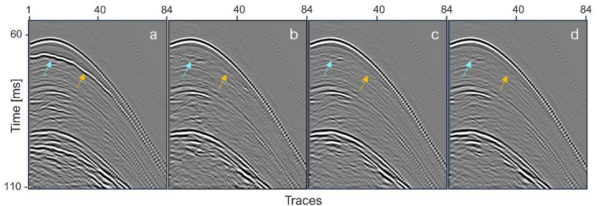
**Figure 1.** Detail of a shot gather before and after deghosting. a) Input with ghost, b) Deghosted with the  $\tau - p$  method, which is used to generate ground truth data, c) Deghosted with the conventional DL, d) Deghosted with the ACL-DL method.
