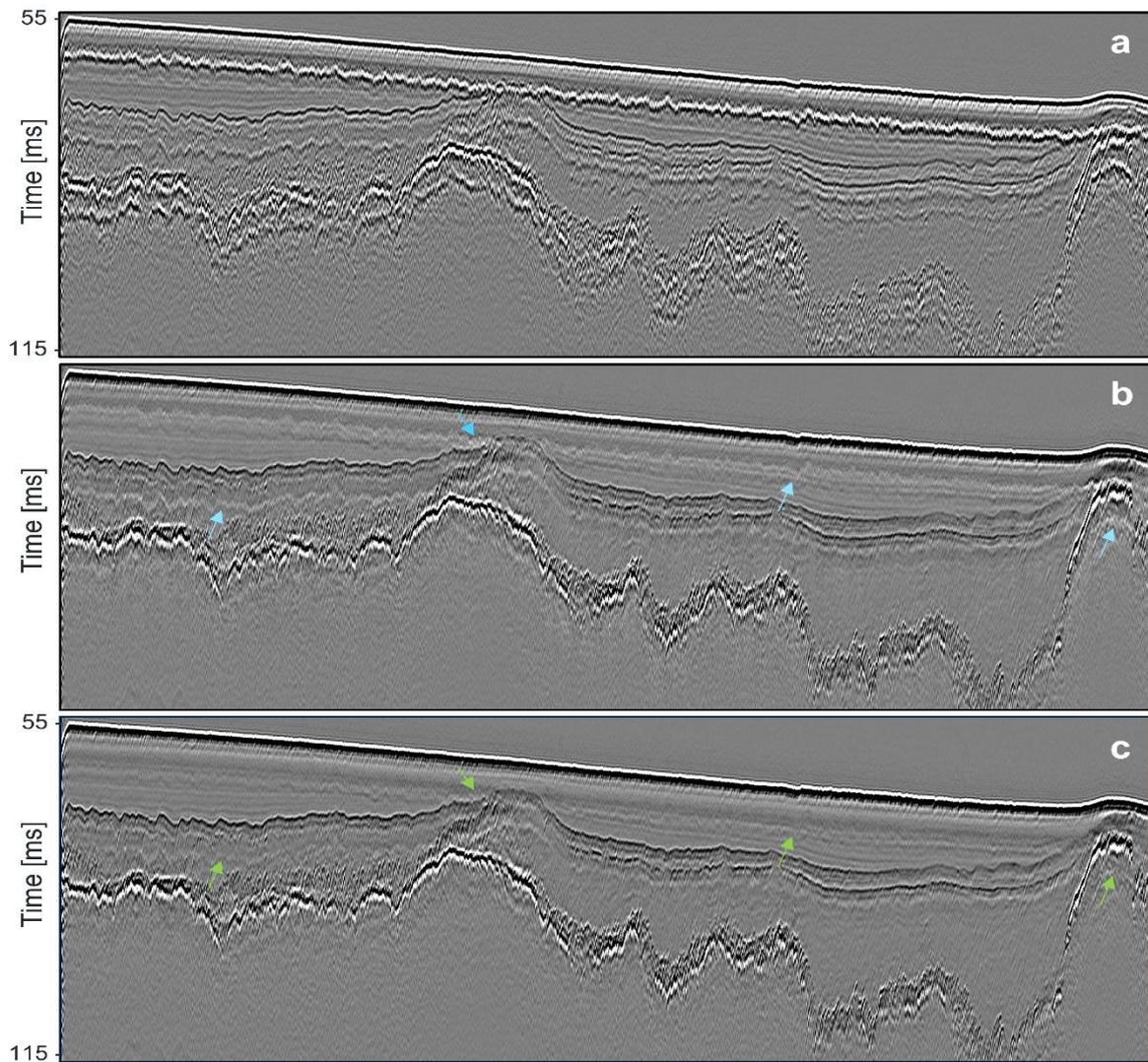
**Figure 3.** Full QC stacked line before and after deghosting. a) Input before deghosting, b) output after the conventional DL deghosting method, c) output after the ACL-DL deghosting method.
