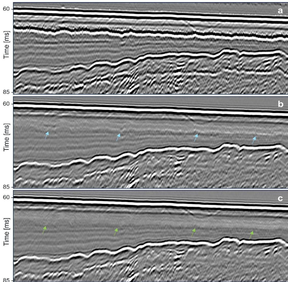
**Figure 2.** Detail of a QC stacked line before and after deghosting. a) Input before deghosting, b) output after the conventional DL deghosting method, c) output after the ACL-DL deghosting method.
