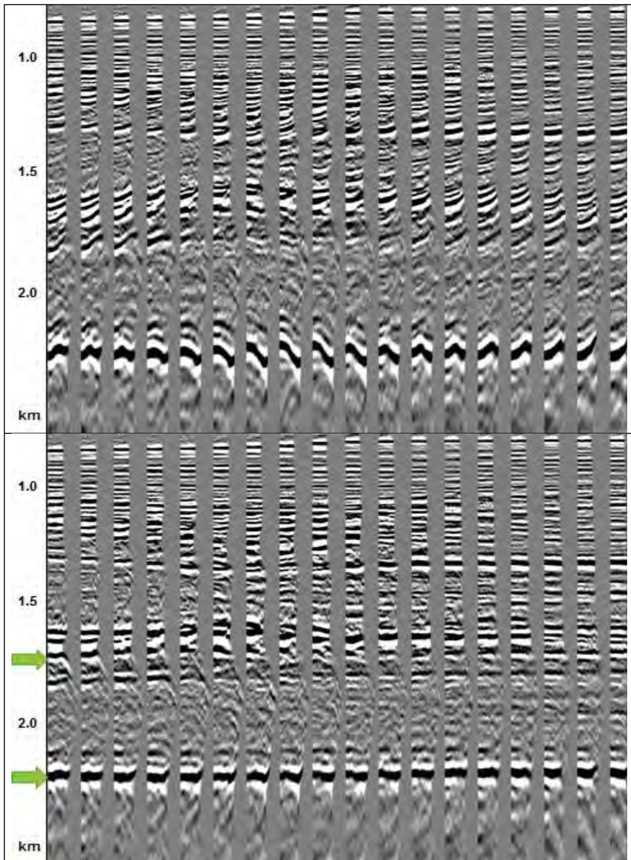
**Figure 3** Top: 3D PreSDM CRP gathers in the zone below the paleo-canyon complexity after several iterations of parametric picking (5km maximum offset). Bottom: After four iterations of non-parametric moveout picking, the result is improved. Overall CRP gather flatness is significantly improved for these deeper major reflectors.
