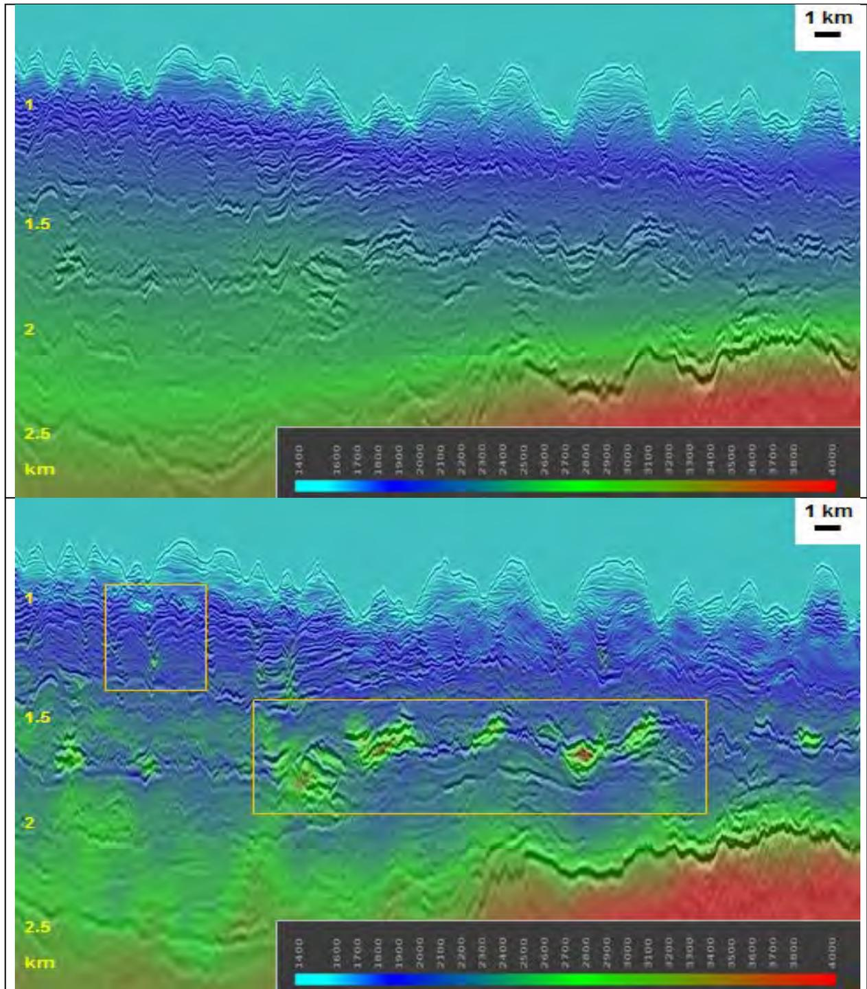
**Figure 4** Top: Final Kirchhoff 3D PreSDM image in the zone below the paleo-canyon complexity after several iterations of parametric picking, with interval velocity overlay. Bottom: Corresponding image after four iterations of non-parametric (generalised) moveout picking. The boxes indicate areas where higher resolution velocity information has been recovered. Overall the image is improved for all deeper major reflectors.
