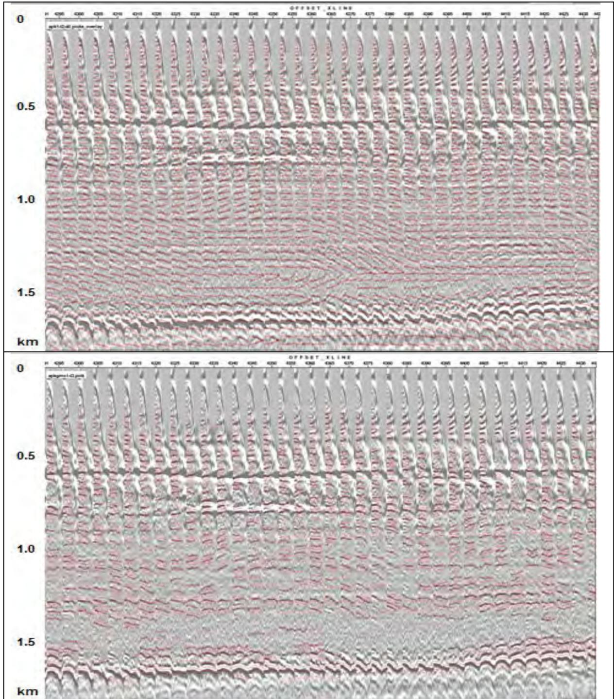
**Figure 8** Top: 2<sup>nd</sup> order parametric pick (red lines) superimposed on the final set of gathers from the conventional update based on parametric picking. Bottom: Non-parametric picking of the same gathers. The ‘V’ and ‘n’ shaped moveout behaviour of the gathers for the deeper reflector are well-tracked by the non-parametric autopicker.
