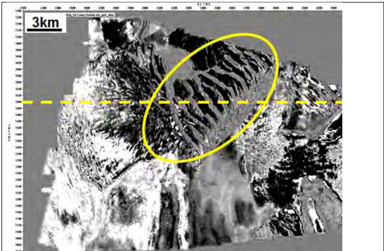
*Figure 6 Slice at 800m through low-velocity eroded layer. The ellipse highlights the eroded region, and the dashed line indicates where Figure 5 intersects the feature.*
