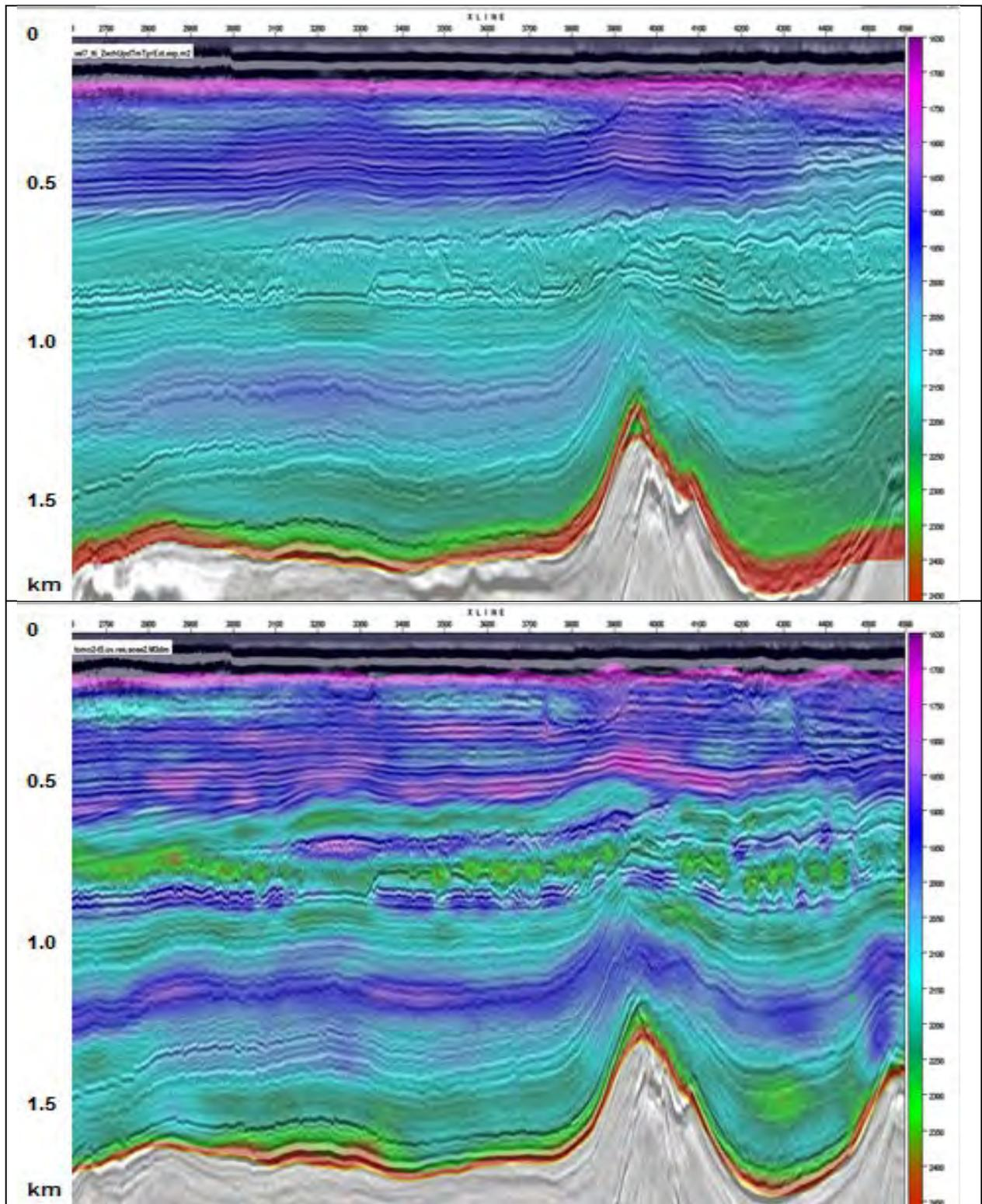
**Figure 10.** Final 3D PreSDM images with colour velocity overlay for the gathers shown in Figure 9. Top: After 2<sup>nd</sup> order parametric picking and update. Bottom: After non-parametric picking and update.
