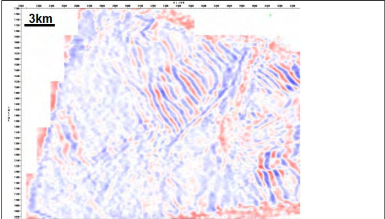
**Figure 7** 2<sup>nd</sup> order parabolic residual velocity error autopicked from muted gathers on a 50m\*50m CPR grid.
