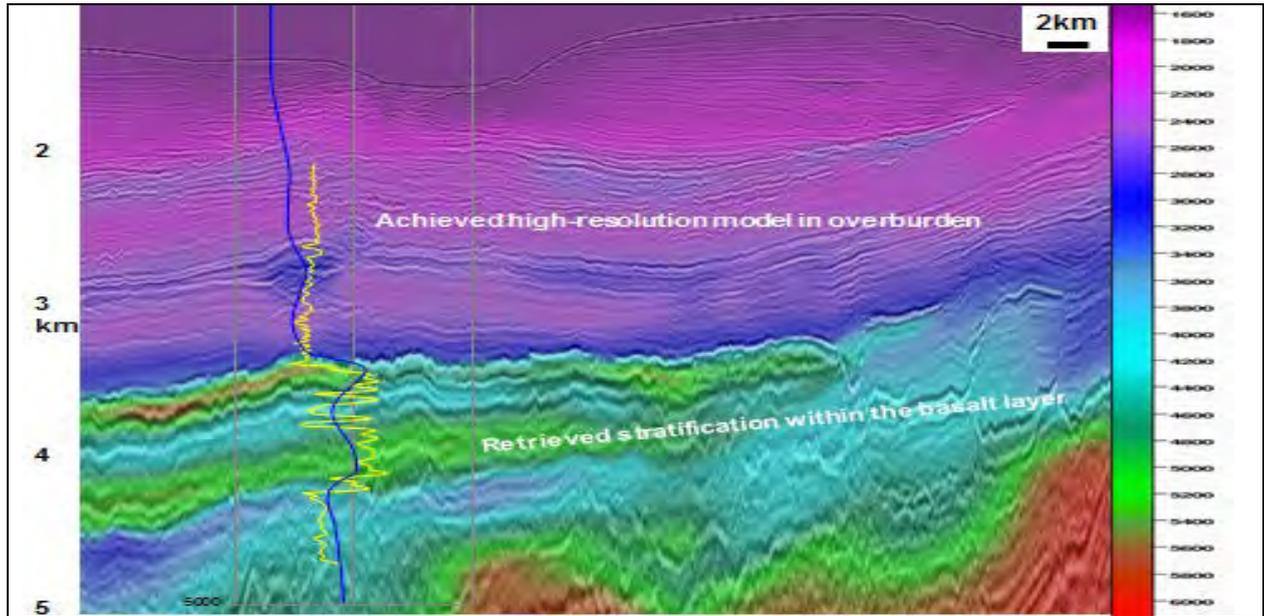
**Figure 1** For the vast majority of the study area, parametric picking and inversion worked well. Hi-resolution tomographic inversion was able to resolve layering within the basalt and identify trapped sediment units in the basal flows.
