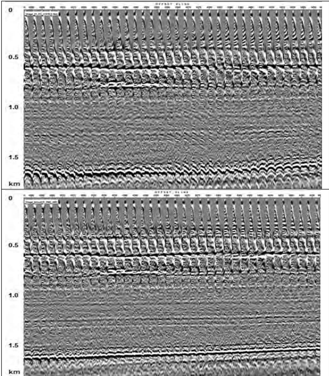
*Figure 9 Top: CRP gathers after 2<sup>nd</sup> order parametric picking and update (as shown in Figure 8). Bottom: CRP gathers after non-parametric picking and update, showing well-flattened gathers.*
