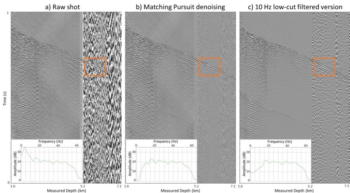
**Figure 4** A sample raw shot a) before and b) after Matching Pursuit flow noise attenuation. c) The application of a conventional denoising process. Amplitude spectra of the selected area (orange) are also compared at the bottom of each figure.
