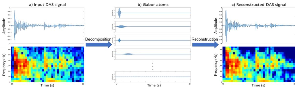
**Figure 2** The decomposition and reconstruction of a field DAS signal obtained by Matching Pursuit.
