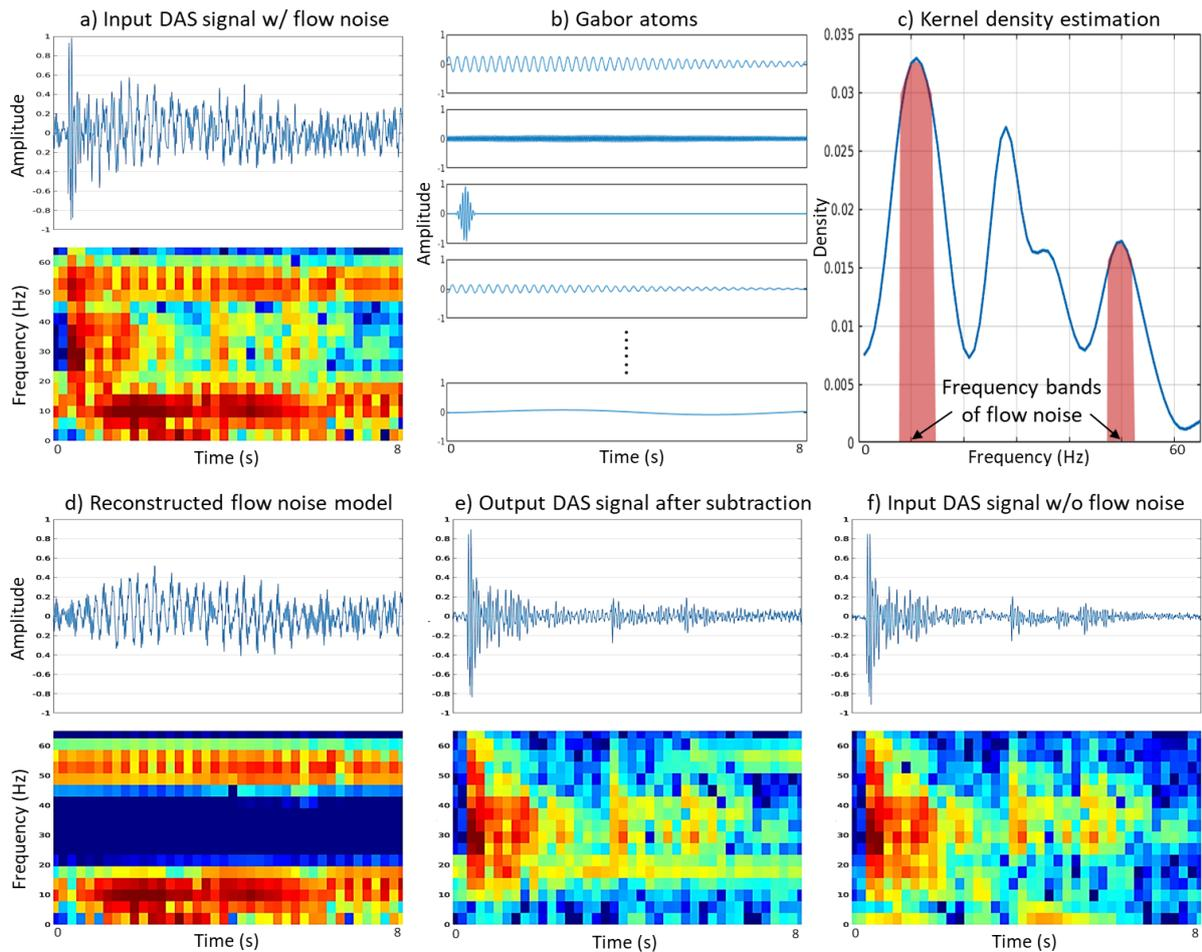
**Figure 3** Illustrations of flow noise attenuation workflow based on Matching Pursuit.
