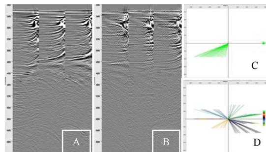
Figure 6: (a) CMP gathers from a common source-receiver pair; (b) 3D CMP gathers; (c) Offset azimuth distribution for (a); (d) offset-azimuth distribution for (b).
