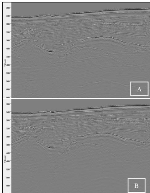
Figure 4: Stacked data without (a) and with (b) 3D SRME.
