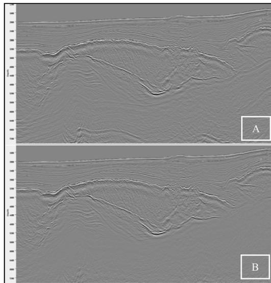
Figure 5: 2D PreSTM data without (a) and with (b) WFE.
