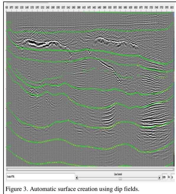
Figure 3. Automatic surface creation using dip fields.
