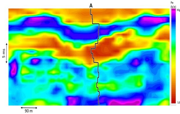
Figure 8: Segment of Pe section passing through blind well A. Pe curve is overlain on the Pe section for comparison.
