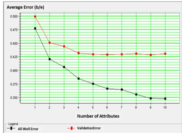
Figure 4: Average training and validation error versus number of attributes for the optimum operator length of 7 samples. Black curve represents average training error and red curve represents average validation error. The validation error does not improve after 5 attributes.
