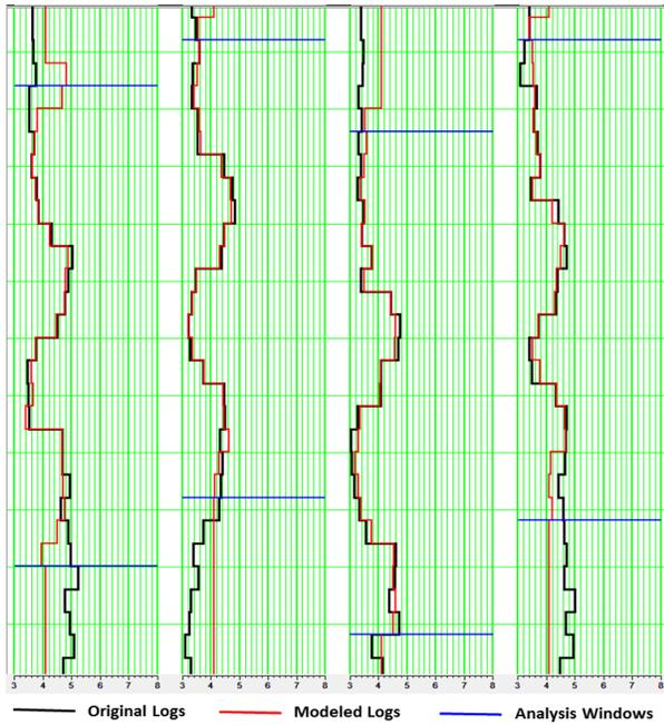
Figure 7: Log panel showing the match between actual Pe log and modeled Pe log derived using PNN for different wells.
