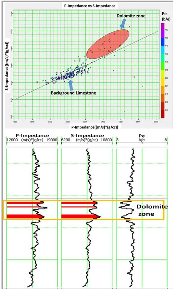
Figure 2: Crossplot of well log P-impedance and S-impedance, color coded with Pe log curve (above). Captured points enclosed by the red polygon are back projected on the well log panel (below).
