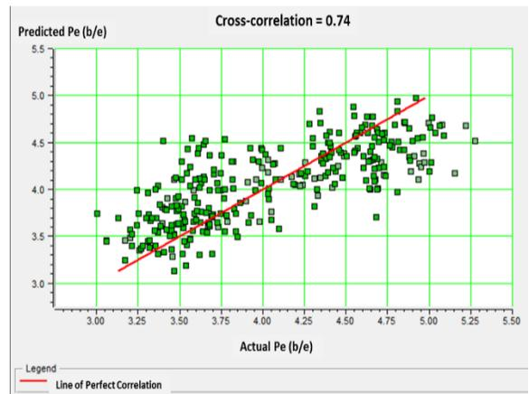
Figure 5: Crossplot of actual Pe and predicted Pe derived using multiattribute linear regression for 12 wells. A correlation of 0.74 is observed between actual and predicted Pe.
