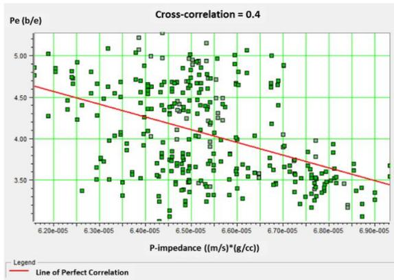
Figure 3: Crossplot of inverted P-impedance and well log Pe for 12 wells. A correlation of only 0.4 is observed between inverted P-impedance and well log Pe.
