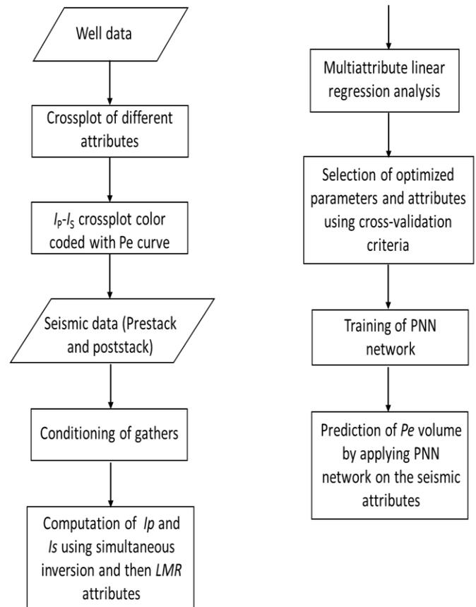
Figure 1: Integrated workflow for estimating Pe volume to characterize the dolomite reservoir
