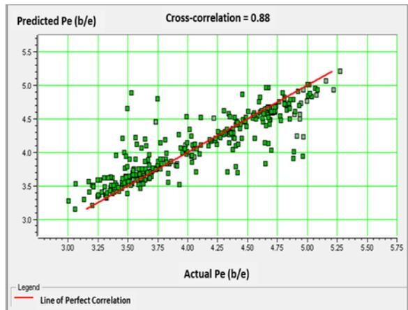
Figure 6: Crossplot of actual Pe and predicted Pe derived using PNN for 12 wells. A good correlation of 0.88 is observed between actual and predicted Pe.
