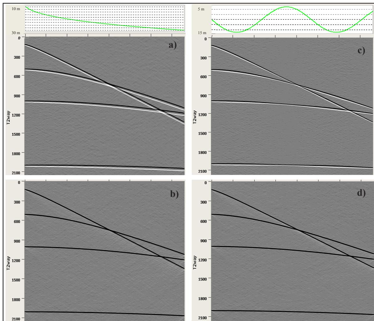
**Figure 4** a) A synthetic shot gather conformed of four events associated with their receiver side ghosts generated assuming a parabolic streamer shape. b) After redatuming and deghosting while acknowledging the depth of every individual receiver. c) A synthetic shot gather generated assuming a sinusoidal streamer shape. d) After redatuming and deghosting. Note that b) and d) are quite similar as expected.
