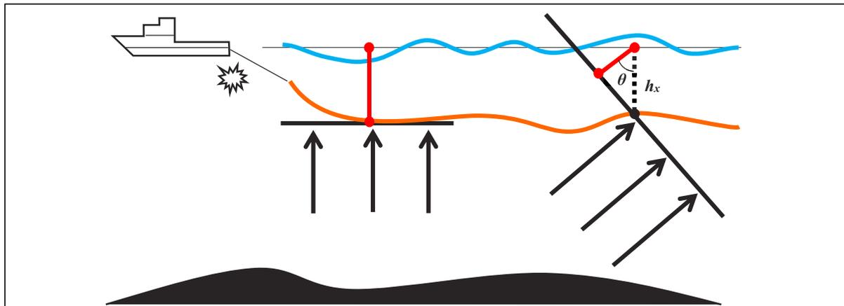
**Figure 2** Schematic diagram of redatuming seismic wavefields recorded by a curved streamer to the Mean Sea Level. A time shift of  $h_x \cos \theta / v_w$  acknowledges both elevation of every individual receiver, and the angle of each plane-wave component. Every slowness trace is obtained via slant-stacking, after redatuming all contributing traces accordingly.
