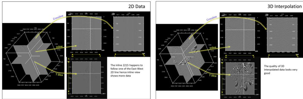
Figure 6. (Left) input 2D data binned into 3D grid and (Right) after interpolation
