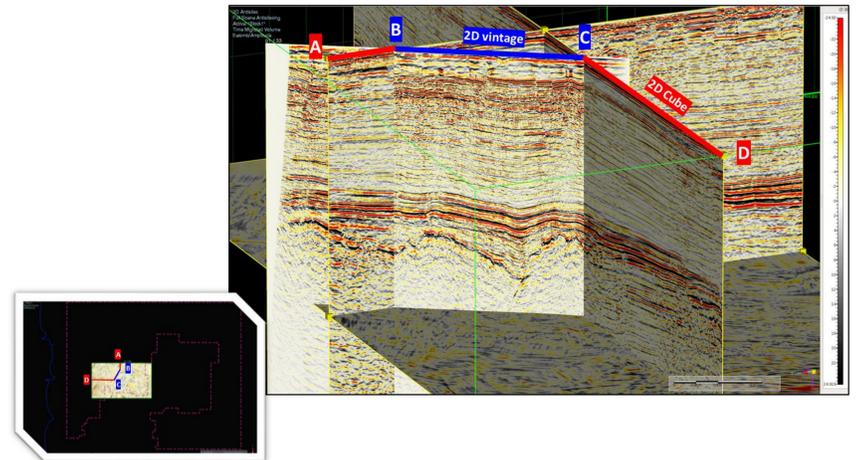
Figure 10. 3D display showing good correlation between existing 2D vintage data and output 2D<sup>cubed</sup> data
