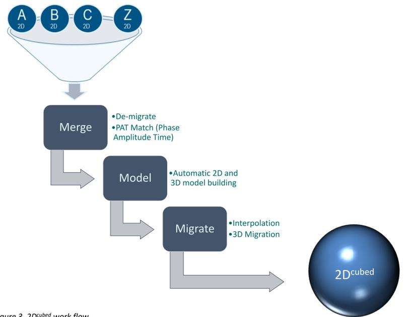
Figure 3. 2D<sup>cubed</sup> work flow
