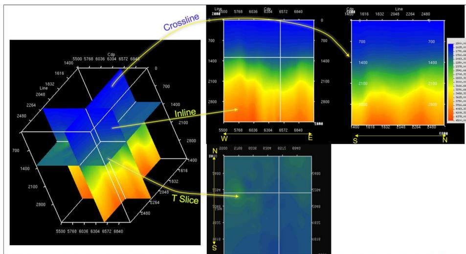
Figure 7. 3D Velocity model used in 3D poststack migration
