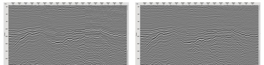
Figure 4. Oblique Line display before and after survey matching.
