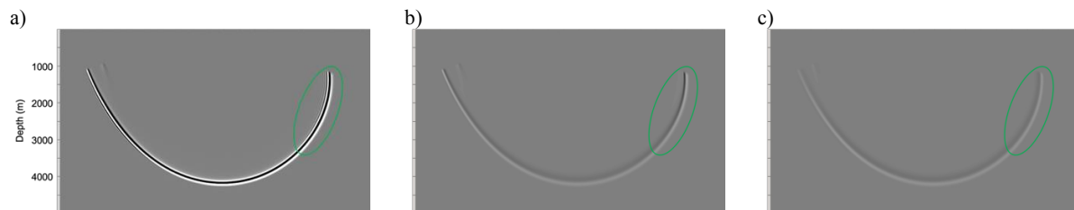
Figure 1: Comparison of wavefield snapshots without attenuation in (a), with attenuation only in the thin-lens term in (b), and with the proposed method in equation 6 in (c). An angle mute at 75^\circ has been applied to all these snapshots. Here, the angle is measured from the line between the source and the point.
