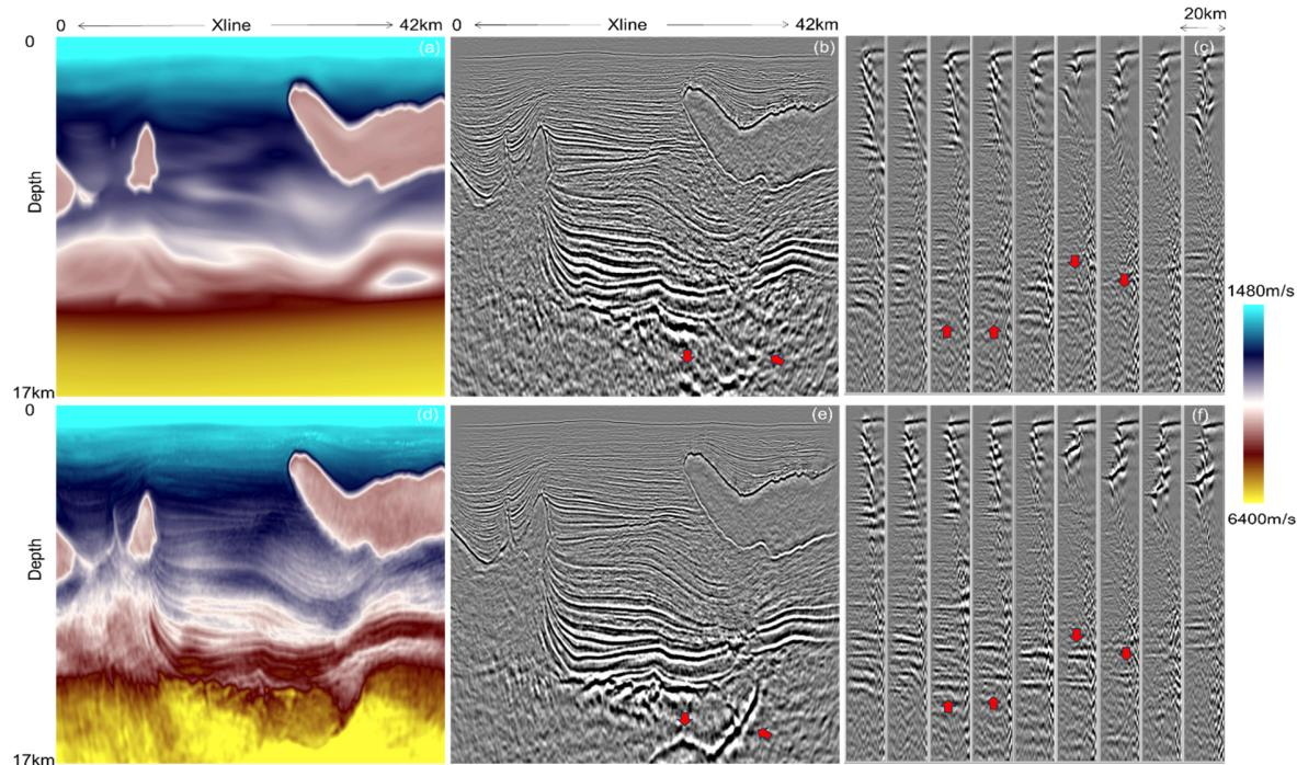
Figure 4: Crossline velocity model, migration image and gather with initial model (a)(b)(c) and FWI velocity model (d) (e) (f)
