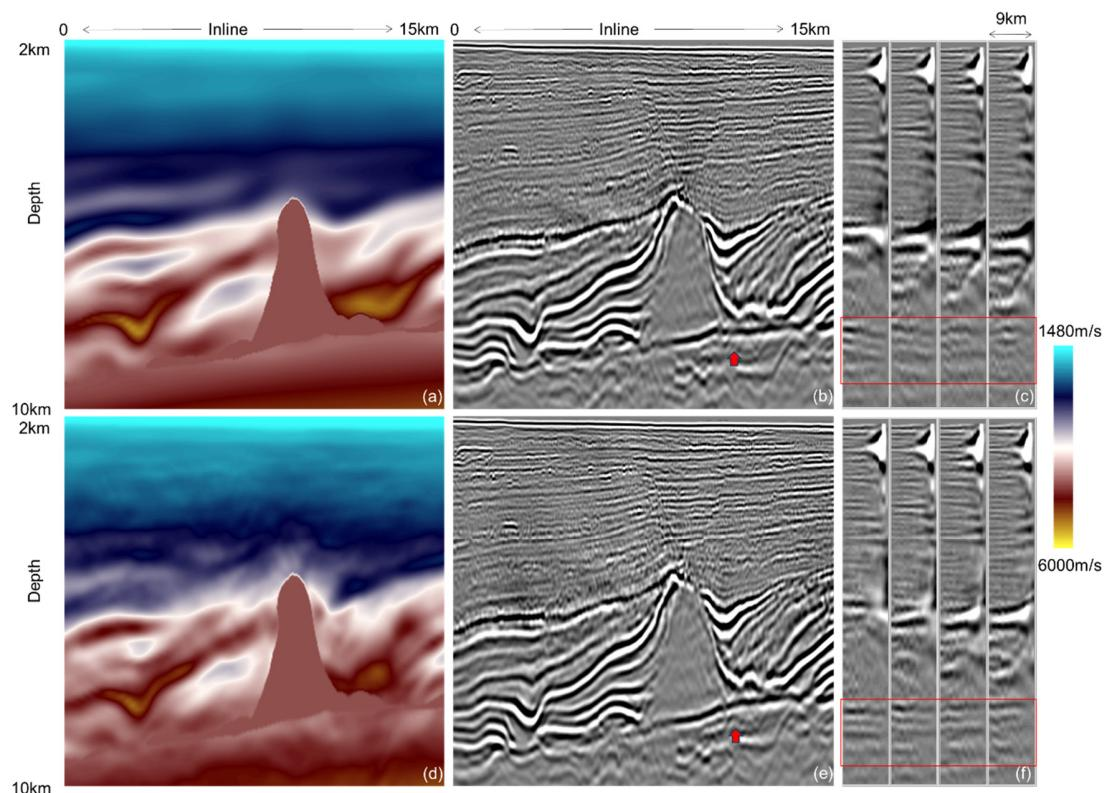
Figure 1: Velocity model, migration image and gather with initial model (a)(b)(c) and FWI velocity model (d) (e) (f)
