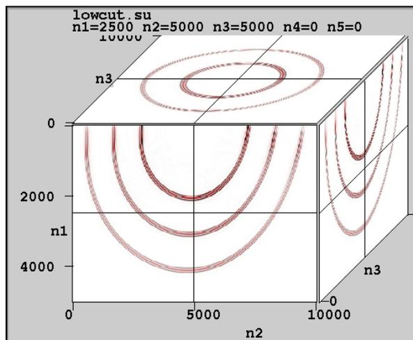
Figure 2: RTM impulse response of a tilted-orthorhombic homogeneous model.
