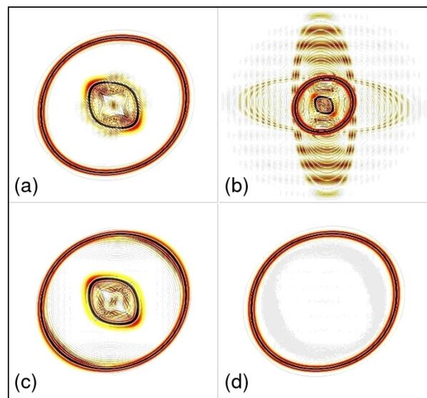
Figure 1: Wavefield snapshot of a homogeneous orthorhombic model using (a) direct finite-difference implementation of equation (1), (b) self-adjoint first-derivative implementation by centered finite-difference, (c) self-adjoint first-derivative implementation by staggered finite-difference without wavefield interpolation, (d) selective damping with equation (7).
