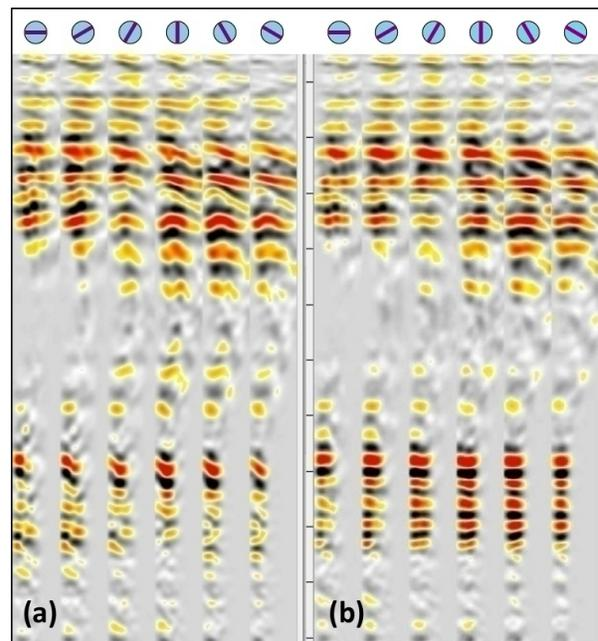
Figure 4: Azimuth-angle gather comparison between (a) TTI and (b) orthorhombic RTM.
