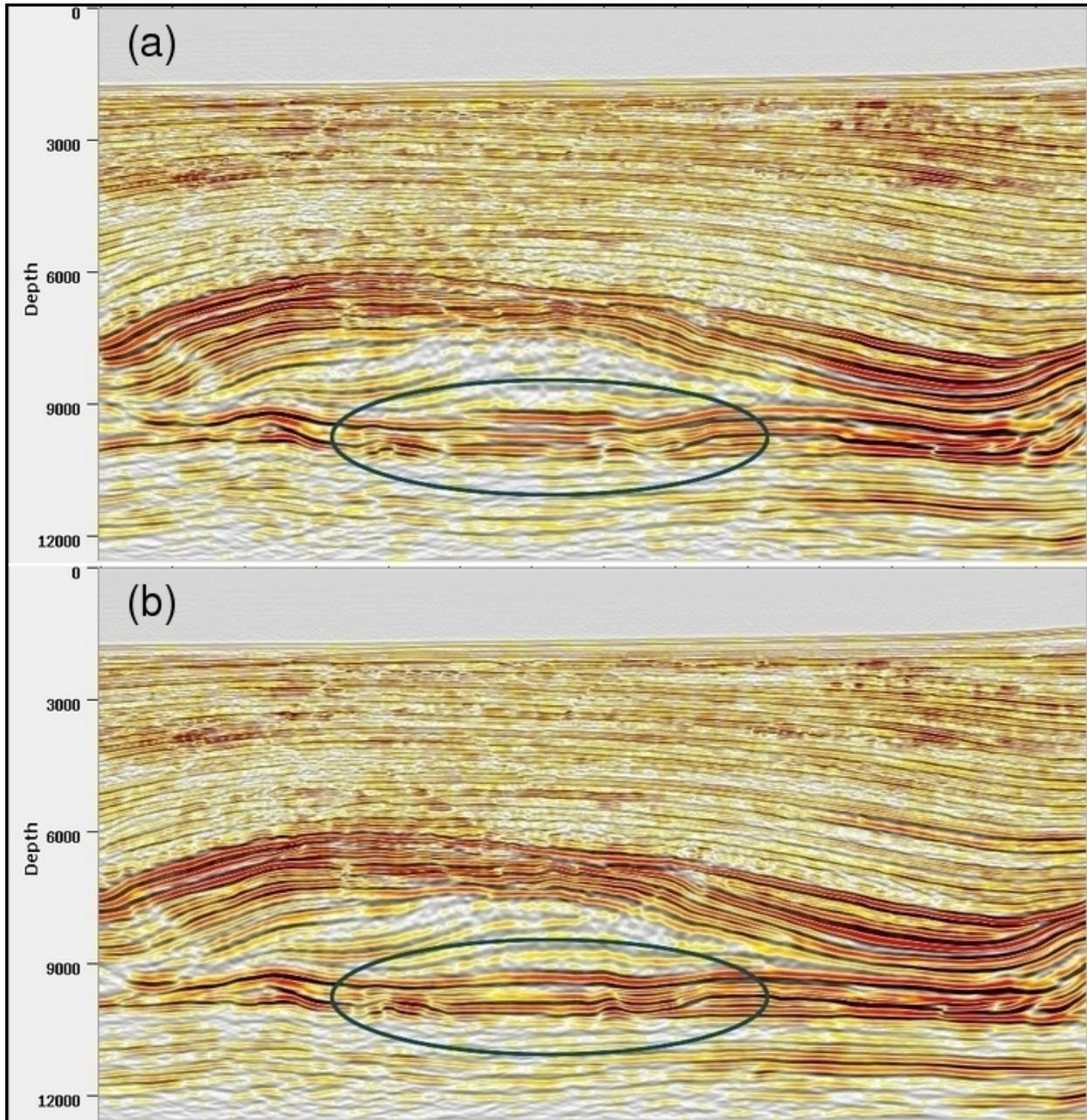
Figure 3: A comparison of (a) TTI RTM and (b) orthorhombic RTM images.
