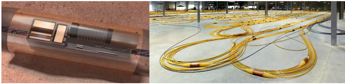
Figure 2 4C sensor station and cable during system integration and SIT.
