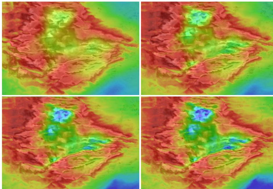
**Figure 4** Seismic depth slice at 585m with the FWI velocities overlaid. Initial model from wavelet shift tomography (top left), 2-6Hz FWI model (top right), 2-10Hz FWI model (bottom left), and 2-14Hz FWI model (bottom right).
