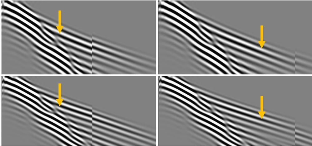
**Figure 3** Comparison at mid- and far offset of synthetic shot points before and after velocity scaling. Anisotropy was kept fixed in the examples shown in the top row. The same comparison with fixed velocity and anisotropy parameters adjusted below BCU is shown in the bottom.
