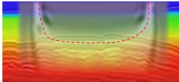
**Figure 1** Seismic image of a shallow target structure with its interval velocity model overlaid. An illustration of a forward modelled, 2-6Hz diving wave has been superimposed on the plot. The white event (highlighted with a red, dashed line) represents the wave propagation. The source to receiver offset for the modelled wave is 6km and the depth range shown is from 0 to 1.5km.
