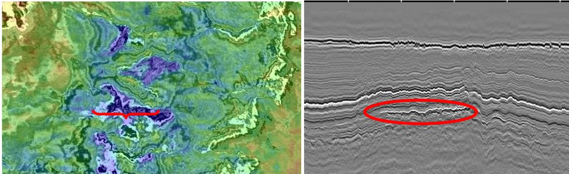
**Figure 5** Depth slice of the FWI model overlaid on the corresponding reflection image (left). Subline image thought the anomaly (right). The red ellipse high-lights the bright spot that correlates to the low velocity zone in the FWI model.
