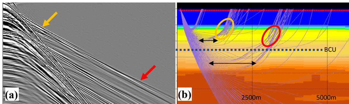
**Figure 2** Shot record from the survey (a) showing the two main refracted events. The second event (red arrow) propagates into the BCU and can be tracked over a large offset range. Ray tracing results superimposed on the FWI model (b). The two main refractors are marked by ellipses.
