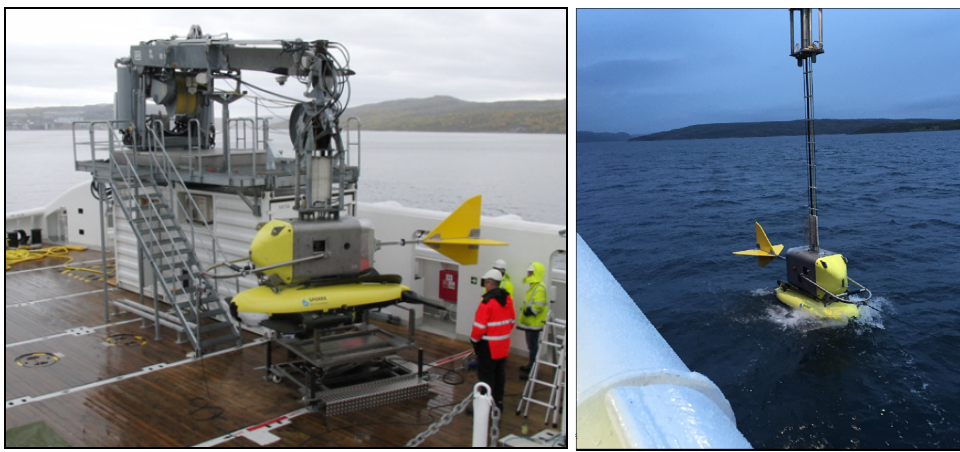
Figure 3 The ROST ready for deployment by the Launch and Recovery System (left) and during deployment at forward speed (right).
