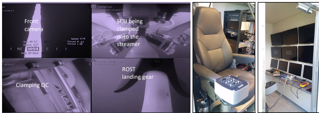
Figure 4 Left: An example of ROST control screen. Middle: Pilot co-pilot chair. Right: ROST control monitors.
