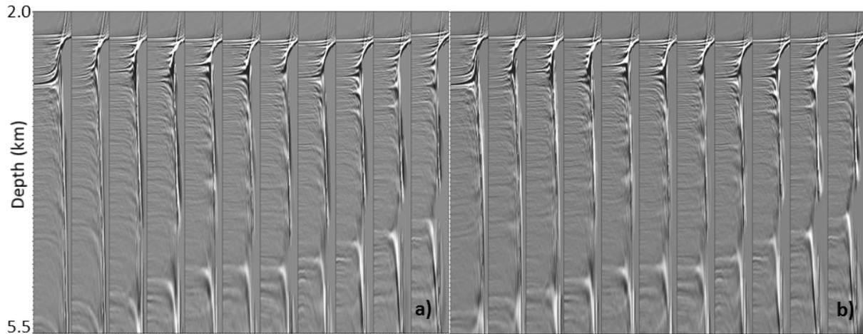
Figure 3. Kirchhoff image gathers for the a) starting and b) inverted vertical velocity and epsilon models corresponding to the field data example of Gulf of Mexico.
