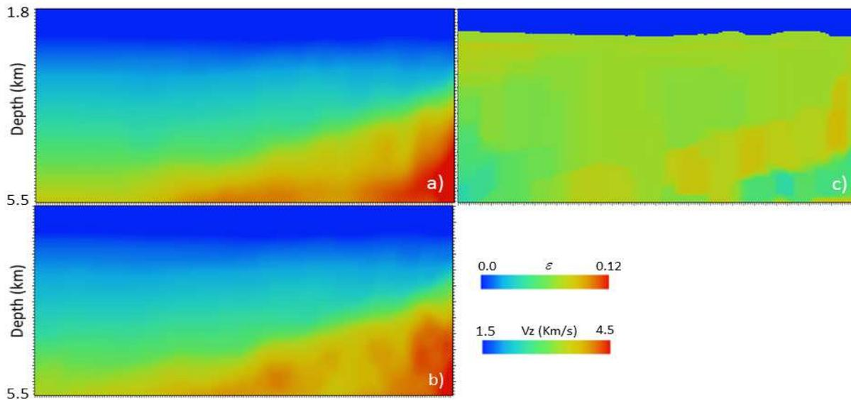
Figure 2. a) Starting vertical velocity model for the Gulf of Mexico field data example; epsilon and delta models are constant from the water bottom and equal to 0,08 and 0.04, respectively. Inverted b) vertical velocity and c) epsilon models after two stages of sequential inversion.
