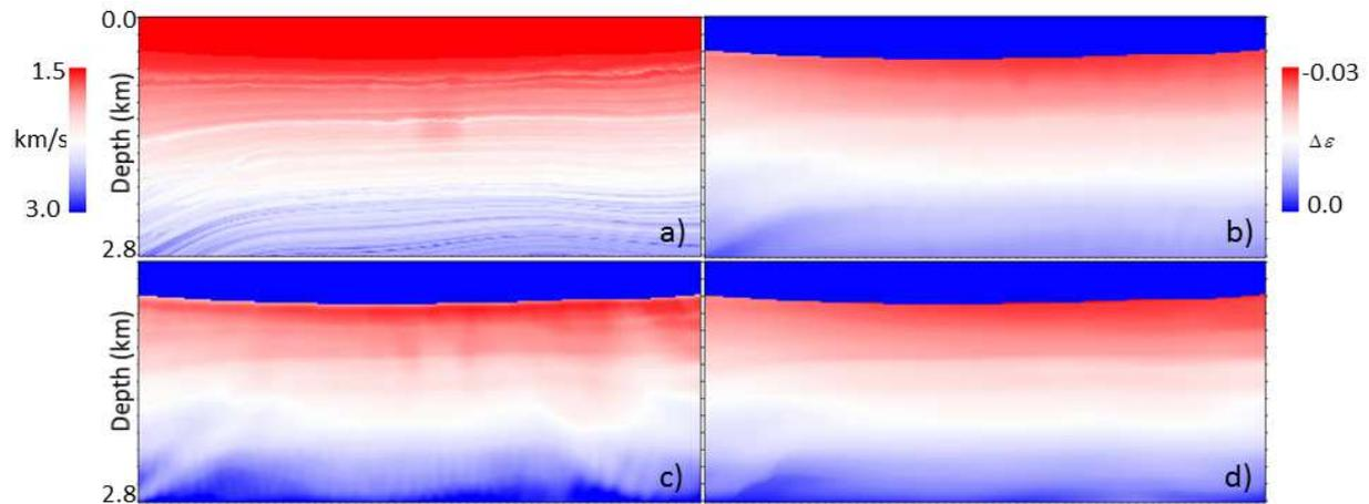
Figure 1. a) Vertical velocity and b) difference between the true and starting epsilon. Epsilon updates after inversion without (c) and with (d) TV regularization.
