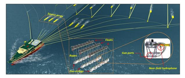
Figure 1 Dual-source configuration. Each source is made of 3 gun strings suspended below floats.
