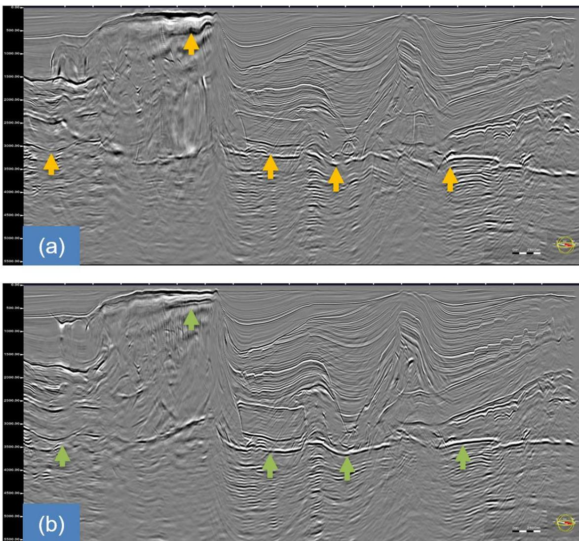
**Figure 3** Inline section of Kirchhoff migration with (a) initial velocity model and (b) the FWI model.
