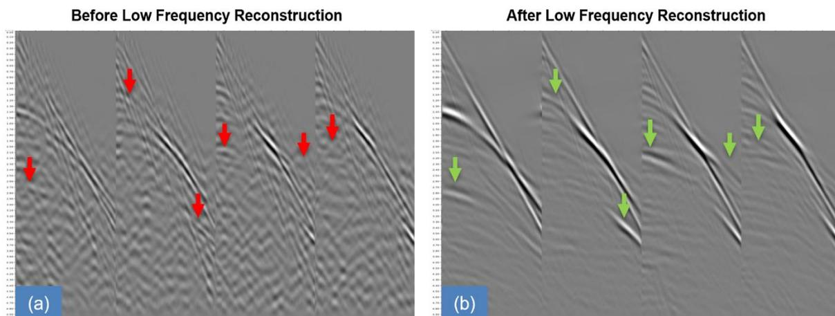
**Figure 1** Shot gathers in the 0-5 Hz band (a) before LFR, (b) after LFR below 4 Hz.
