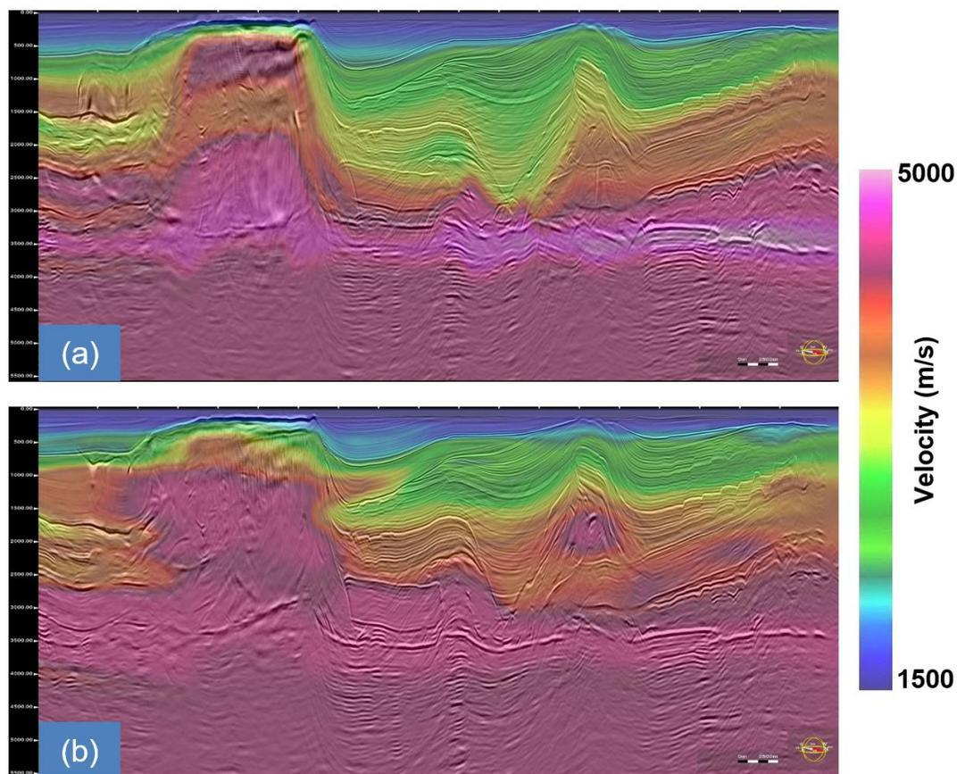
**Figure 2** Velocity models overlaid with Kirchhoff images for (a) the initial model and (b) the FWI final model.
