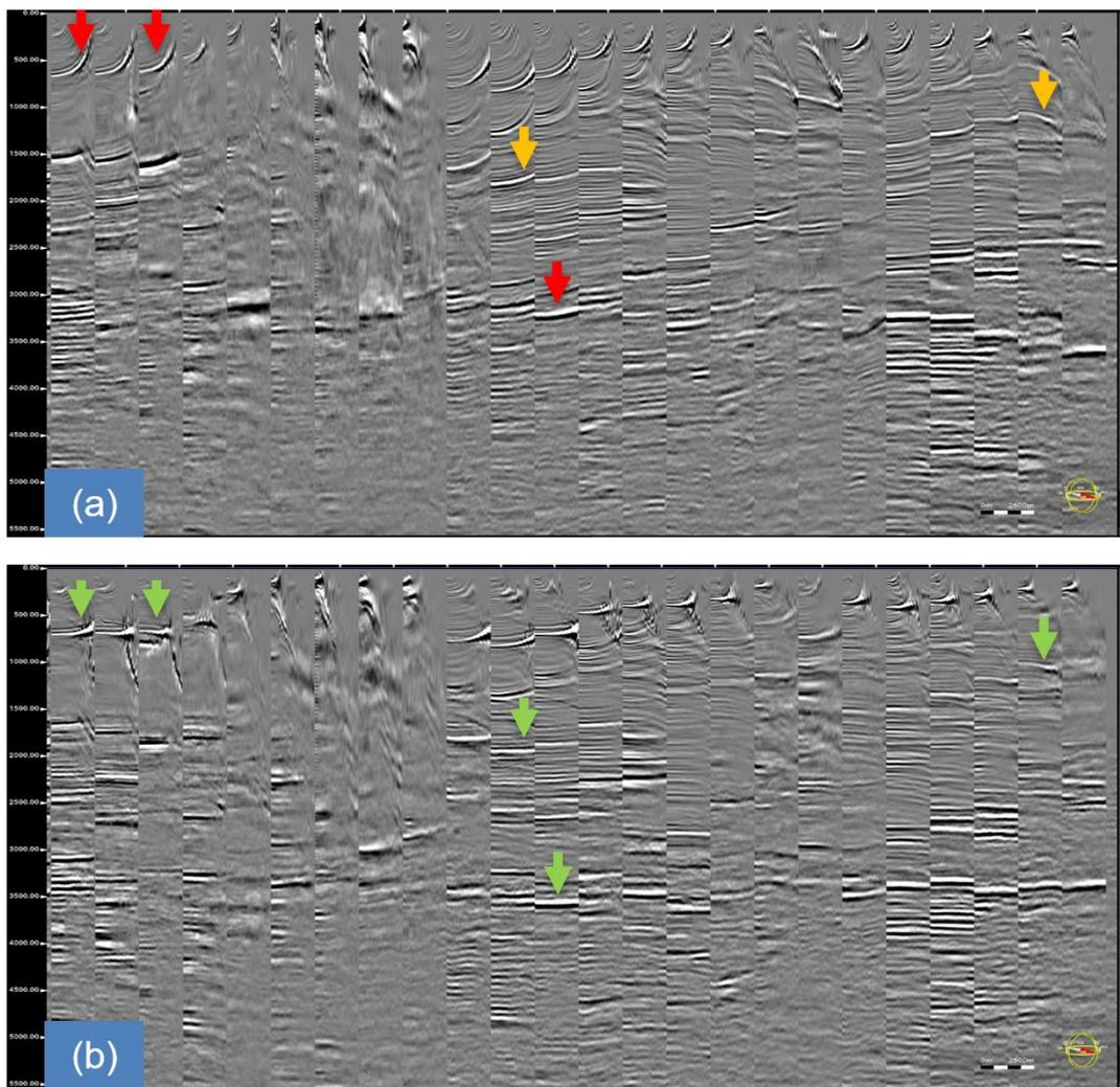
**Figure 4** Inline angle gathers for the Kirchhoff migration with (a) the initial velocity model and (b) the FWI model.
