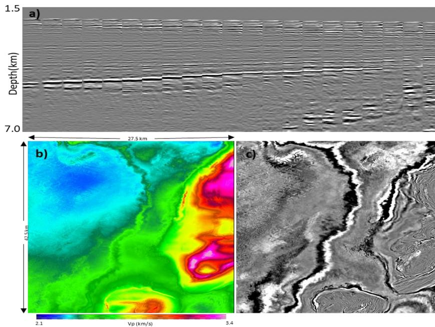
**Figure 4.** Cape Anguille field data. a) Inverted angle-dependent reflectivity along an inline; b) velocity model and c) full stack reflectivity for a depth slice at 3900. The maximum frequency of inversion is 40 Hz.
