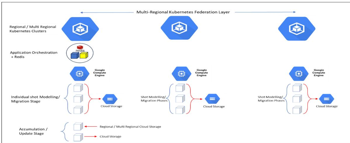
Figure 2. Kubernetes cluster configuration, application partitioning, and fault tolerance aspects of the designed inversion application in the cloud.
