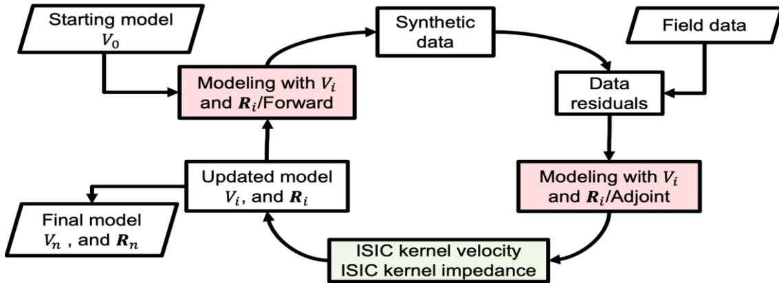
Figure 1. Workflow for simultaneous inversion for velocity and pre-stack reflectivity.
