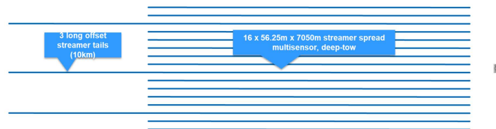
Figure 1 Streamer configuration with sixteen streamers and three streamer-tails for a Barents Sea Survey in 2020 (Widmaier et al., 2021).
