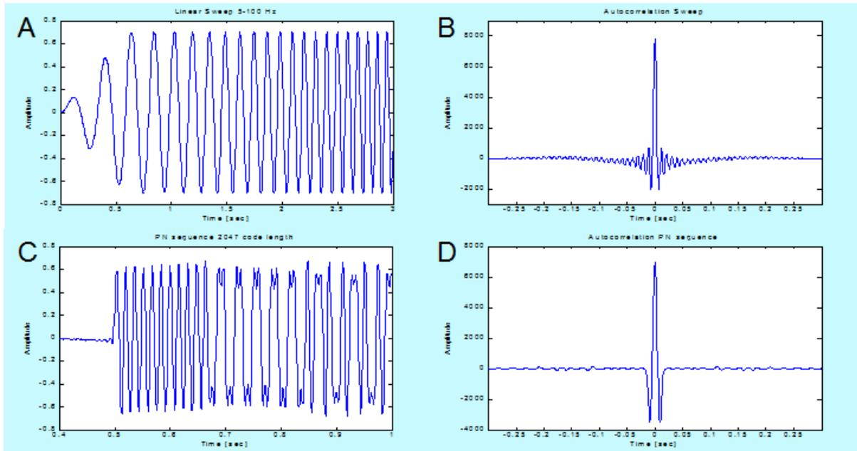
**Figure 2** (A) Linear MV sweep signal; (B) Autocorrelation of A; (C) Spread spectrum MV sweep; and (D) Autocorrelation of C.
