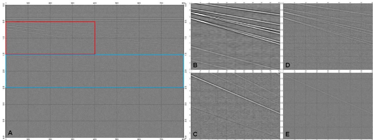
**Figure 4** Synthetic data spread spectrum simulations: (A) 0-4 s synthetic stack generated with the autocorrelation of a 5 s sub-sequence (note the shallow and deep windows used for B-D); (B) 0.5-1.5 s result from a 40 s sub-sequence and 100 m SP interval; (C) 1.5-2.5 s version of B; (D) 0.5-1.5 s result from a 10 s sub-sequence and 12.5 m SP interval; (E) 1.5-2.5 s version of D.
