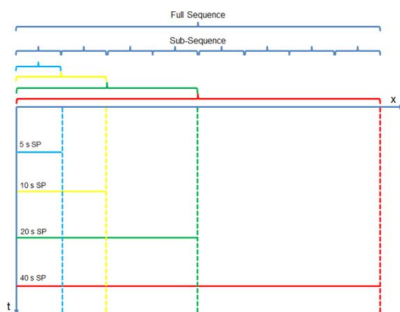
**Figure 3** Spread spectrum sweep strategy: Sub-sequences of varying duration can be selected from the full sequence and used in signal processing to optimize the seismic imaging of different target depth ranges (refer to **Figure 4**).
