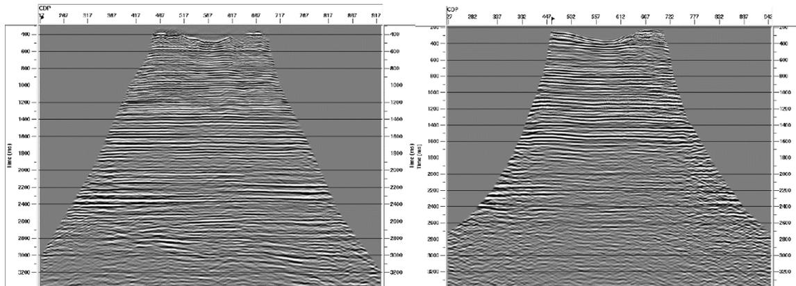
**Figure 5** Stacked sections of the vertical OBC component using an air gun array (left) and spread spectrum marine vibrator sweeps (right). The lines were acquired with different crossline offset to the receiver line, hence the time shift between the sections.
