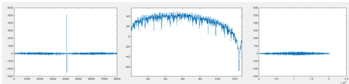
**Figure 1** (left) Autocorrelation of Gold sequence G511a; (middle) Amplitude spectrum for Gold sequence G511a; and (right) Cross-correlation of Gold sequences G511a and G511b.
