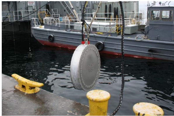
Figure 2 HF module calibrations at Seneca Lake test facility.
