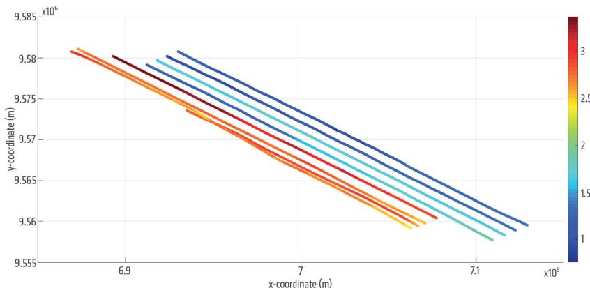
**Figure 5** Vessel locations for the field trial with bottom speed shown in colour.
