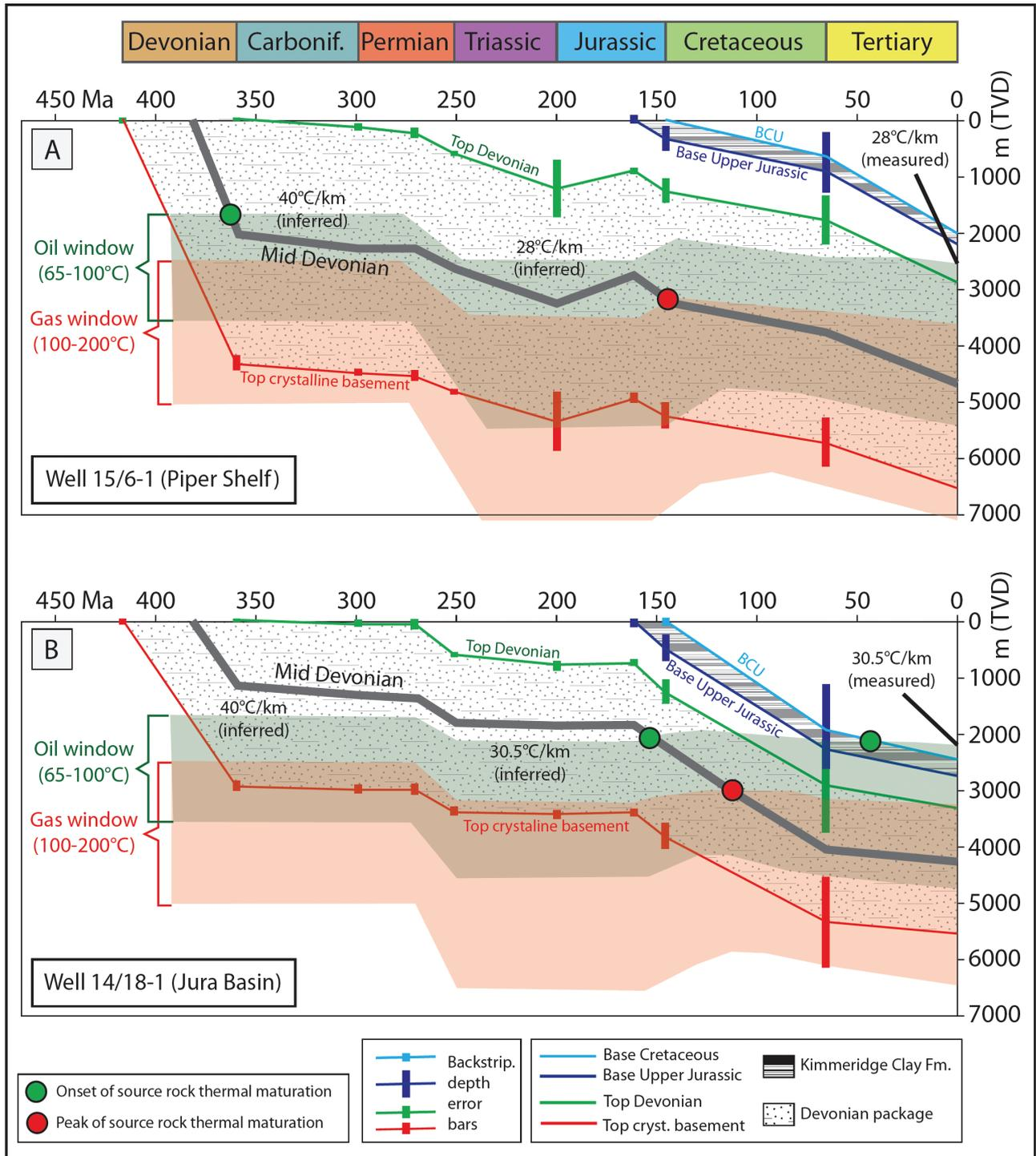
Figure 7 Total subsidence curves below present-day sea level of backstripped wells 15/6-1 (A) and 14/18-1 (B) (method by Allen and Allen, 2005), versus modelled depths of oil and gas maturation windows.
