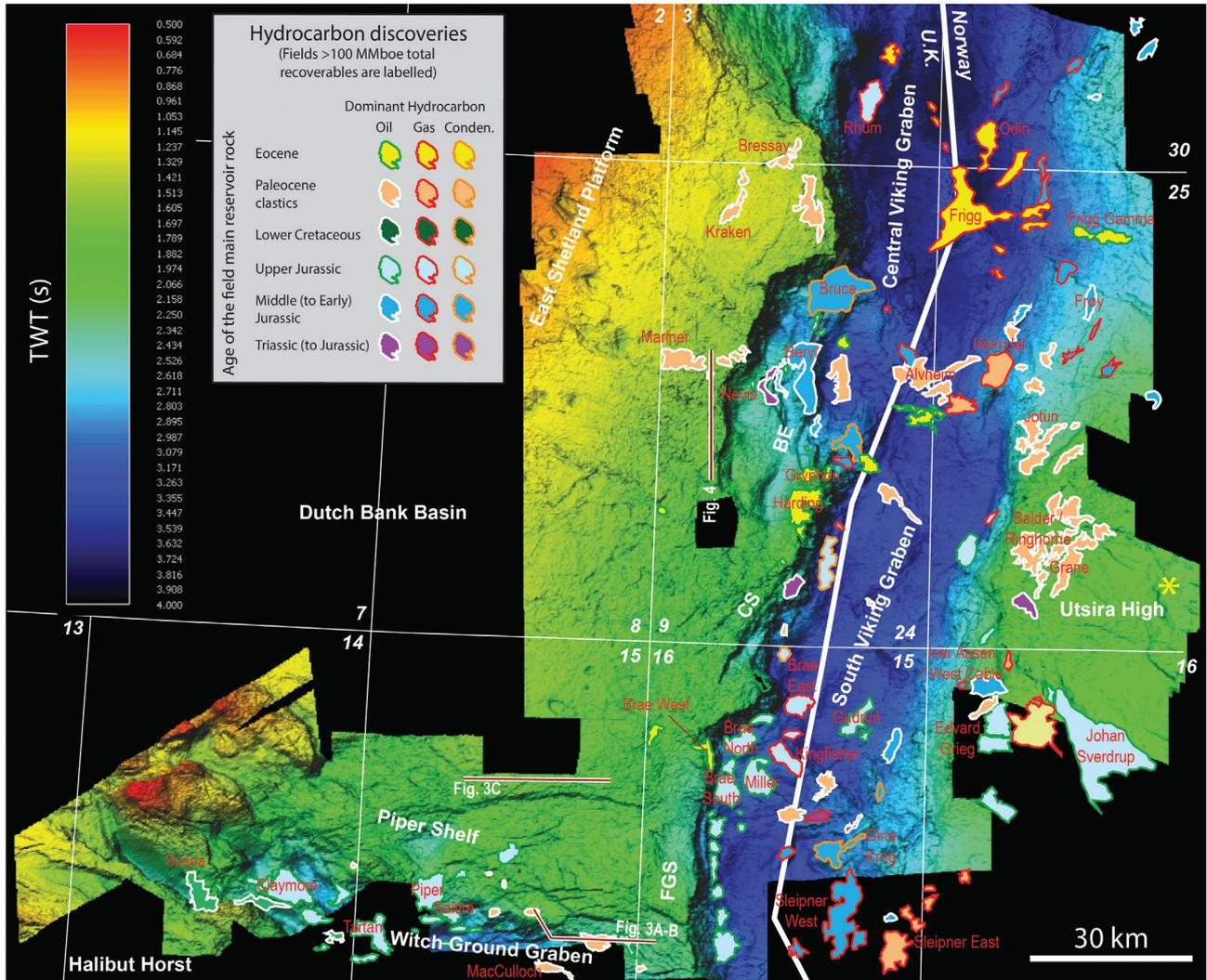
Figure 5 Base Cretaceous Unconformity (BCU) TWT structure map, interpreted on the 9 GeoStreamer 3D surveys highlighted in Figure 1A. The fields and discoveries are also shown, with colours reflecting both the dominant hydrocarbon content and the age of the main reservoir interval. CS = Crawford Spur; FGS = Fladen Ground Spur.
