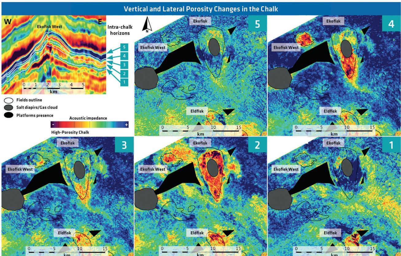
**Figure 7** Amplitude extraction of relative acoustic impedance performed on five intra-Ekofisk horizons. Abrupt changes of chalk porosity, vertically and spatially, are well imaged by the broadband dual-sensor data. Observe the good match of low acoustic impedance (red)/high-porosity/chalk with field outlines.
