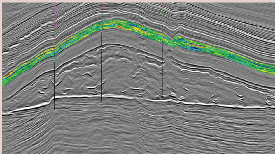
Figure 2. Seismically derived porosity over the BC 28 structure in the SNS Vision dataset allows a 3D understanding of the distribution of aquifer parameters which can be utilized directly in geological modeling and more sophisticated volumetric calculations beyond simple equations.
