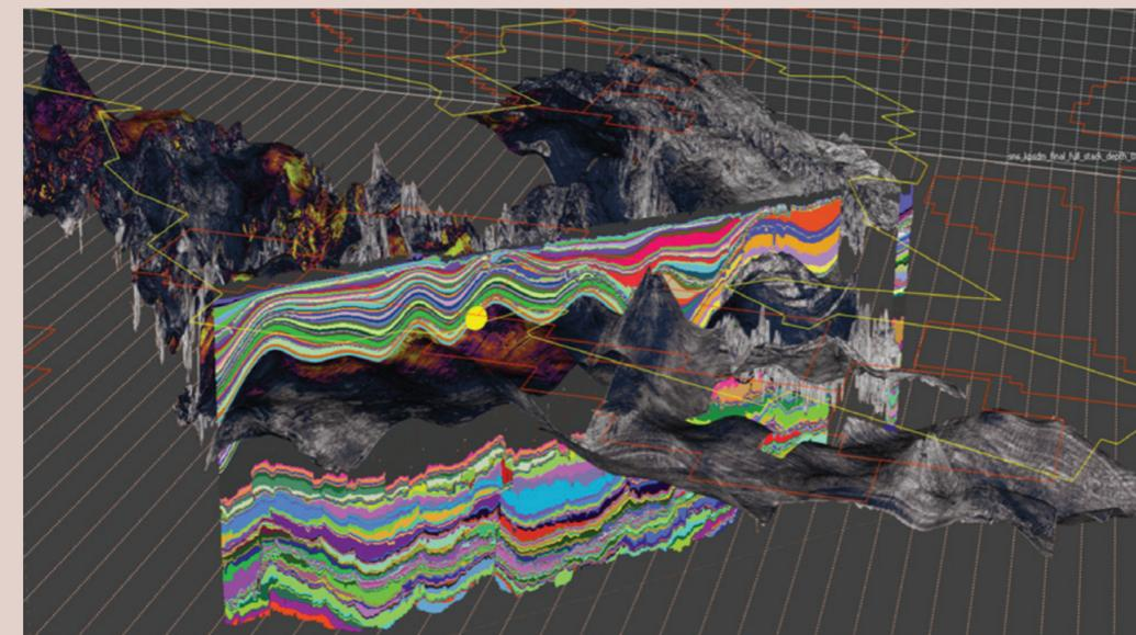
Figure 4. 3D representation of the Relative Geological Time model and the top of the salt over the 12 000 km<sup>2</sup> of reprocessed seismic data. The internal salt structure has been excluded from the seismic interpretation and the focus has been on the top and base salt. Interpretation RGT model produced using Ellis PaleoScan with PGS data.
