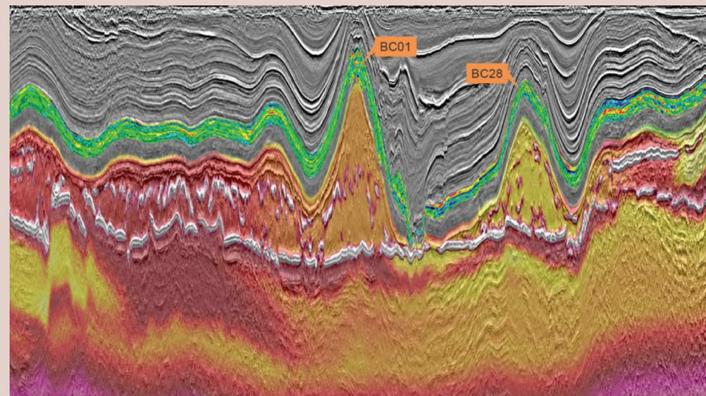
Figure 3. Seismic cross-section through PGS' SNS Vision data illustrating a co-rendering of the final PSDM stack, estimated porosity for the Bunter Sandstone Formation and the seismic velocity.
