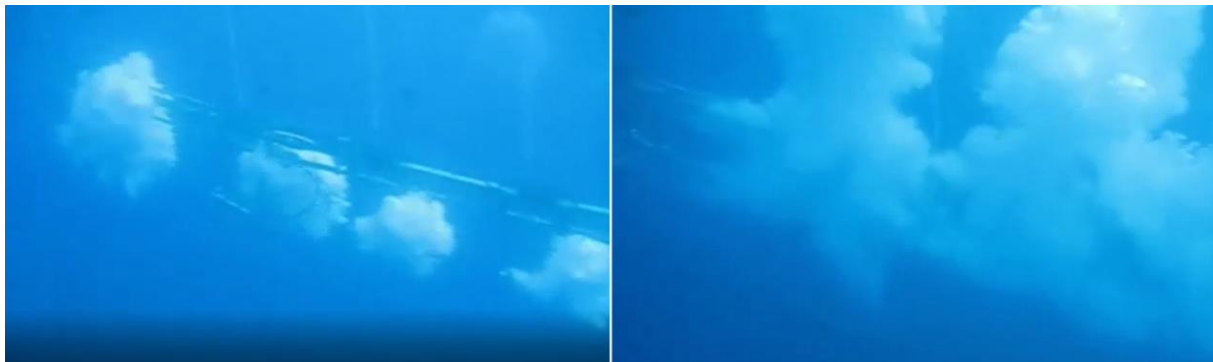
Figure 2. Underwater photo of several air guns being fired. More than 99% of the emitted energy is released within the first 30 milliseconds, with the initial bubble radius being less than 0.5 meters. Thereafter, the air dissipates towards the surface as a benign bubble cloud (right).
