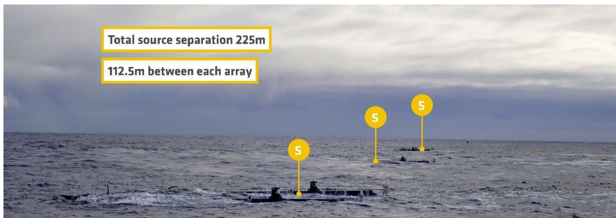
Figure 1: The novel multi-azimuth survey in the Viking Graben used the widest source separation towed by a single streamer vessel on a commercial project to date.
