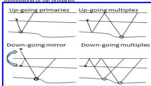
Figure 7 Raypaths for OBS imaging of up-going and down-going wavefields.
