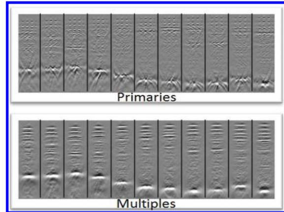
Figure 2. GOM Wide azimuth angle gathers from primaries and multiples with an azimuth 90 degrees from the sail line azimuth. Note the improved angular sampling of multiples.
