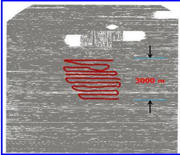
Figure 8. Shown is the configuration of OBS acquisition at Jubarte field - off shore Brazil. The cable layout is show in red and the dense shot distribution is shown in gray.
