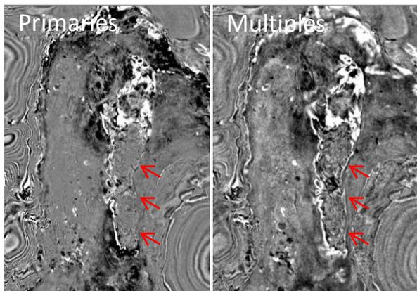
Figure 4. Depth slices at 3km of 3D wide azimuth stack for primaries and multiples. Superior images from multiples over primaries are indicated.
