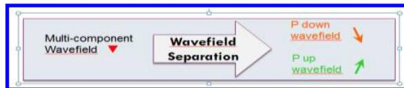
Figure 6. Wavefield separation is used to separate the multi-component data into down and up-going wavefields, which with acoustic approximations, are imaged as compressional waves.
