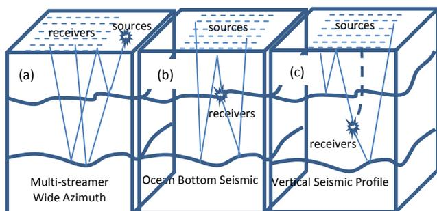
Figure 5. Wide Azimuth Imaging Scenarios: (a) Wide azimuth surface seismic (b) Ocean bottom seismic (c) 3D vertical seismic profiles.
