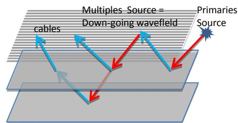
Figure 3. In WAZ acquisition the down-going wavefield in multiples act as a large areal array when compared to a “point” source used in the imaging of primaries.
