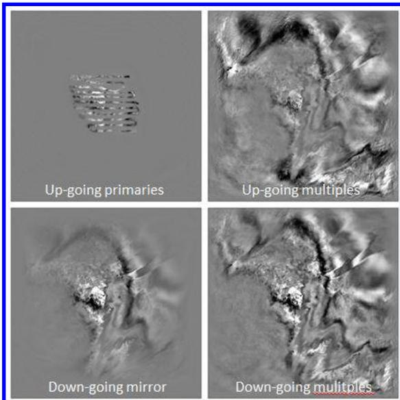
Figure 9 Shown are depth slices of images from up-going primaries, up-going multiples, down-going mirror, and down-going multiples. Note the significant improvement in subsurface illumination from the multiples and mirror reflections over the upgoing primaries.
