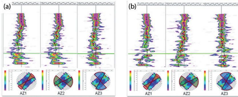
Figure 9 Semblance displays from Kepler three azimuth-sector tomography (a) prior to tomography, and (b) after one pass of azimuth-sector tomography.
