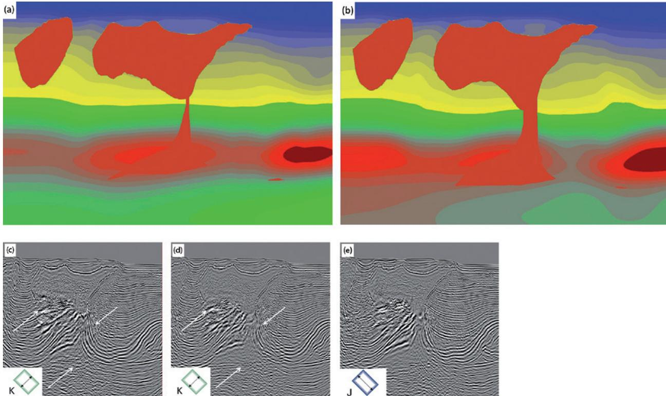
**Figure 12** Results of the test workflows. Final velocity models built on (a) Kepler data only (flow A), and (b) Kepler and Justice data (flow C). RTM migration of (c) Kepler data using the Kepler model only (flow A), (d) Kepler data using the combined Kepler and Justice model (flow C), and (e) Justice data using the combined Kepler and Justice model.
