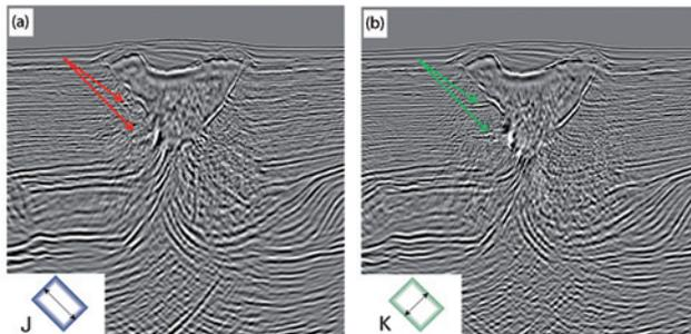
Figure 7 Crossline direction: VTI RTM of (a) Justice survey and (b) Kepler survey. Green and red markers indicate areas of good and poor imaging, respectively.
