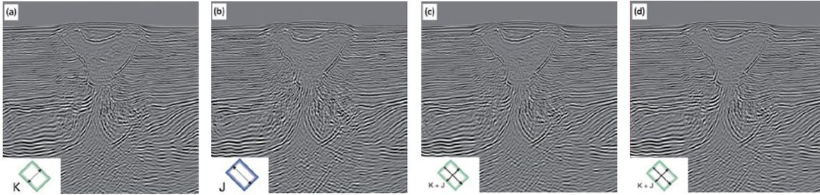
**Figure 14** Final sequence of results for a crossline. (a) Final RTM of Kepler data, (b) Final RTM on Justice data, (c) straight summation of Kepler and Justice, (d) semblance-weighted sum of Kepler and Justice. All migrations used the model from Kepler and Justice data combined.
