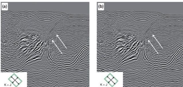
**Figure 13** Final VTI RTM migrations showing (a) straight summation of Kepler and Justice, and (b) summation using semblance-weighted sum. The white arrows indicate a location where the weighted summation has preserved the optimal image from both volumes.
