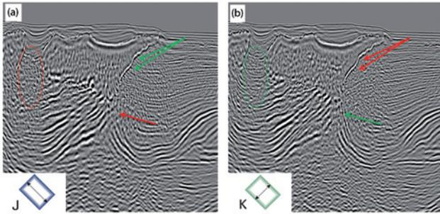
Figure 6 Inline direction: VTI RTM of (a) Justice survey and (b) Kepler survey. Green and red markers indicate areas of good and poor imaging, respectively. The acquisition direction is shown in the inset box in the bottom left corner of each image.
