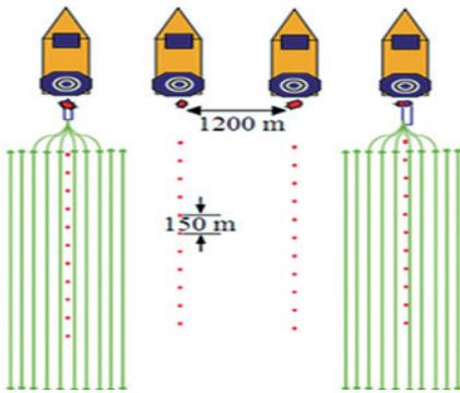
Figure 3 Acquisition set up for the Kepler and Justice surveys.
