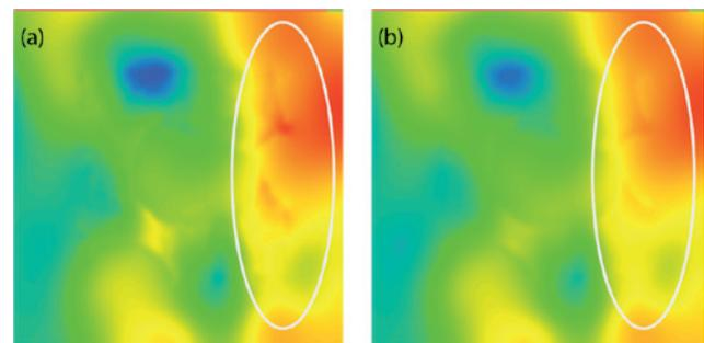
Figure 11 Depth slice at 3600 m after tomography using (a) Kepler survey only, and (b) Kepler plus Justice. The white oval indicates the location of lineations in the Kepler survey attenuated after the six-azimuth tomography.
