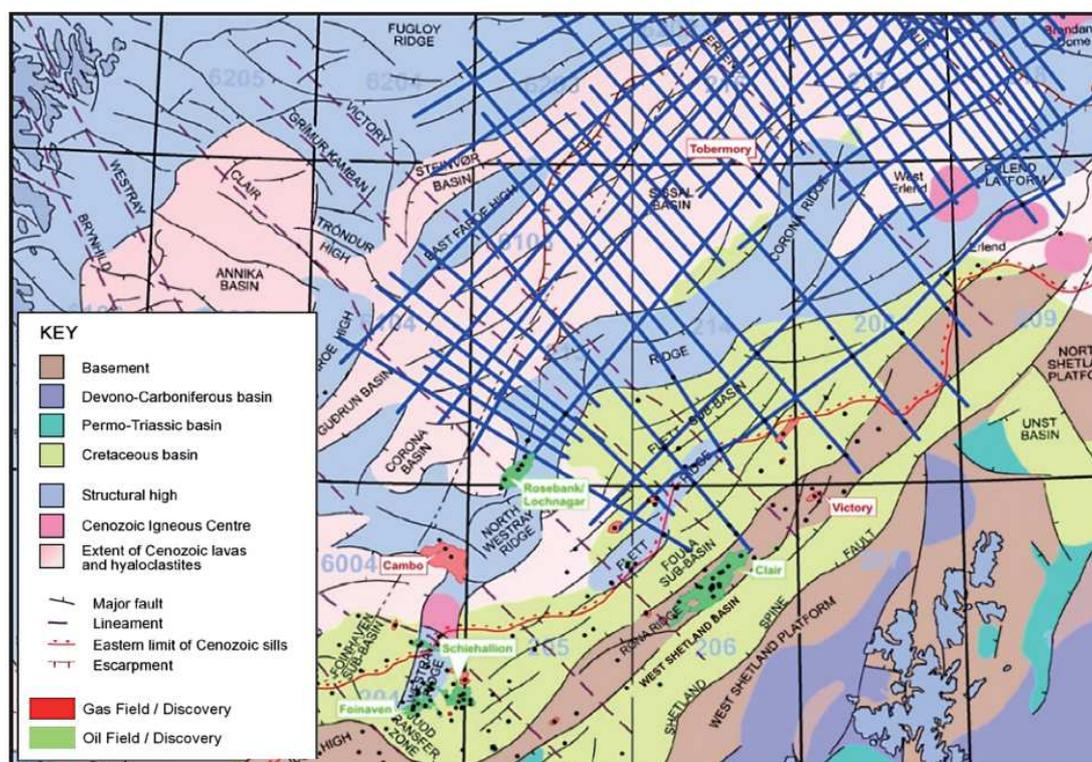
Figure 2: Tectonic elements map of the Faroe-Shetland Basin modified from Moy (2010) showing the reprocessed FSB 1999/2000 2D survey lines in dark blue, wells (in black) and oil/gas discoveries.
