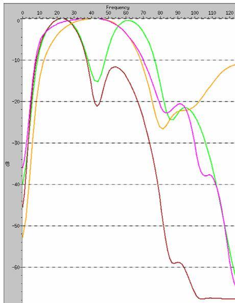
Figure 4: Normalised amplitude spectra of the data derived wavelets shown in figure 3. Green: raw NSR deep tow (fig. 3(a)); Brown: after filter (fig. 3(b)). Orange: FSB 1999 (fig. 3(c)); Pink: FSB 1999 after application of low frequency boosting operator (fig. 3(d)).
