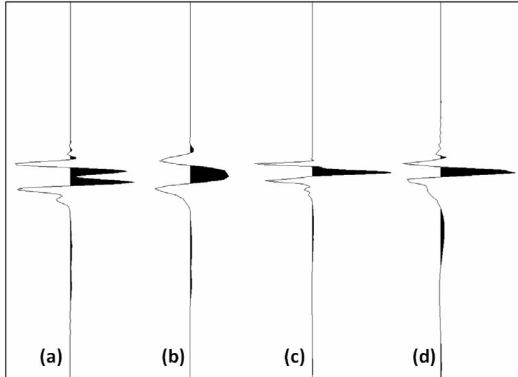
Figure 3: (a) Data derived wavelet from the NSR 2009 18m streamer and (b) after resample to 4ms and 42Hz 36dB/octave high-cut filter; (c) data derived wavelet from the FSB 1999 survey and (d) and spectral manipulation.
