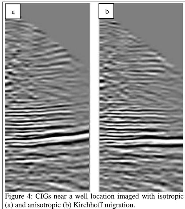
Figure 4: CIGs near a well location imaged with isotropic (a) and anisotropic (b) Kirchhoff migration.
