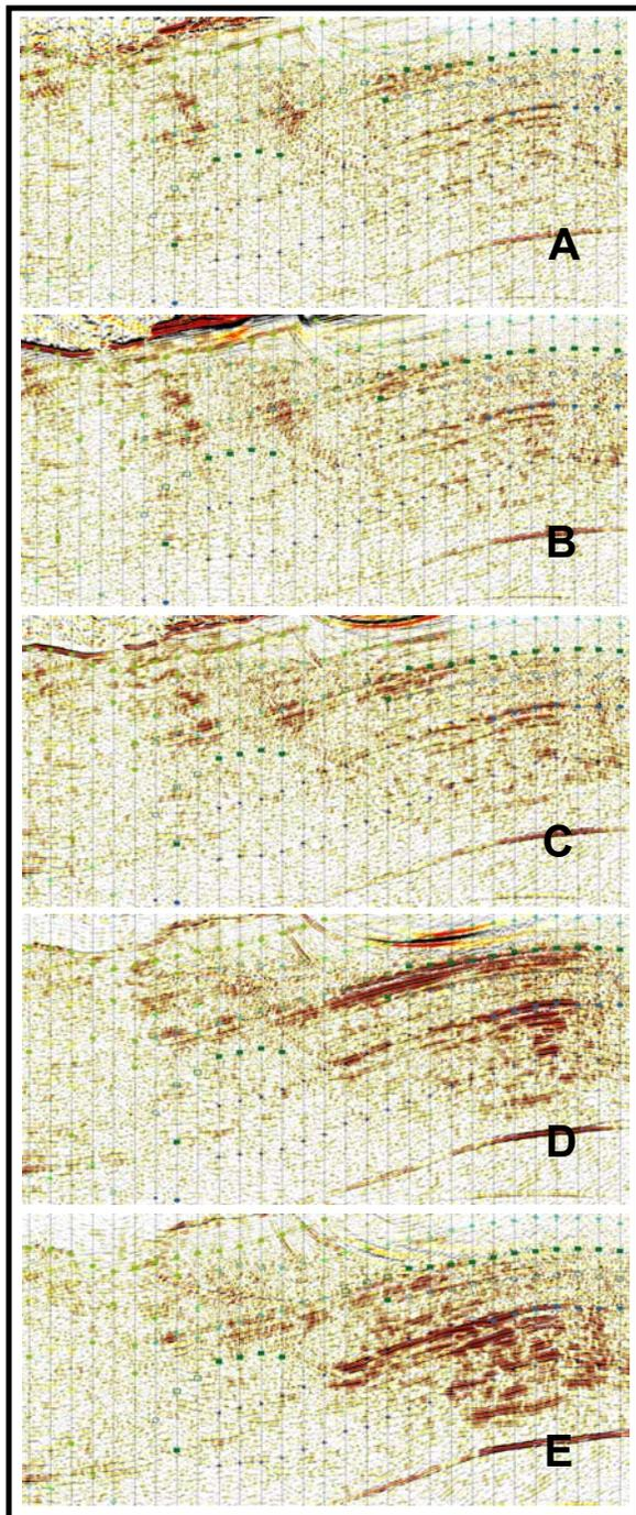
**Figure 2.** A selected RTM-based subsalt DT scan using BP synthetic testing data set: (a) +100 ms; (b) 0 ms; (c) -100 ms; (d) +300 ms; (e) +500 ms.
