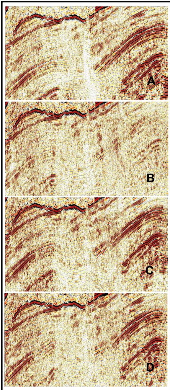
**Figure 4.** (a) RTM images: corresponding to true velocity model; (b) RTM images: corresponding to initial velocity model; (c) RTM composed on DT scan picking corresponding to true velocity model; (d) RTM images: corresponding to updated velocity model;
