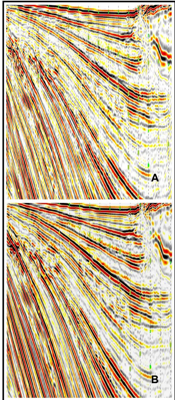
**Figure 5.** 3D real data example of composite RTM image based on DT scan picking. (a) Regular RTM image; (b) Composite image.
