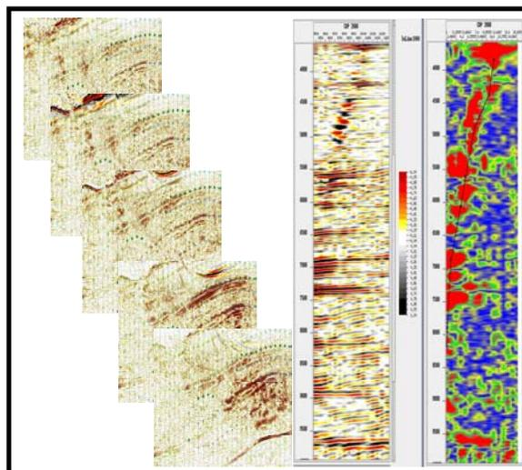
**Figure 1.** An example of RTM-based DT scan in section form (left), gather form (middle), and pseudo-semblance form (right).
