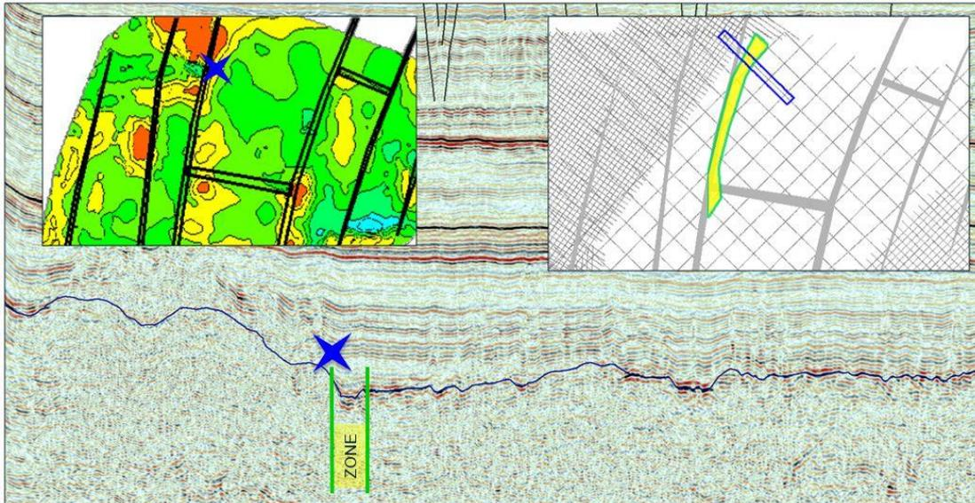
**Figure 2** Transform fault identified on seismic and reviewed on magnetic anomaly map, MGoM. The inset two maps show the VDR transform versions. The blue star indicates the better location of the transform fault, based on the high resolution 2D seismic data. The transform fault zone width is indicated in green/yellow on the seismic and inset basemap.
