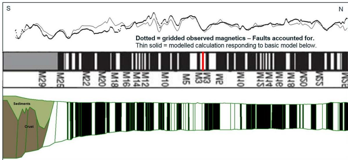
**Figure 4** Forward modelled magnetic profile along a transect in the western most spreading segment in the MGoM (Figure 3), isochron table taken from Walker et al. (2012).
