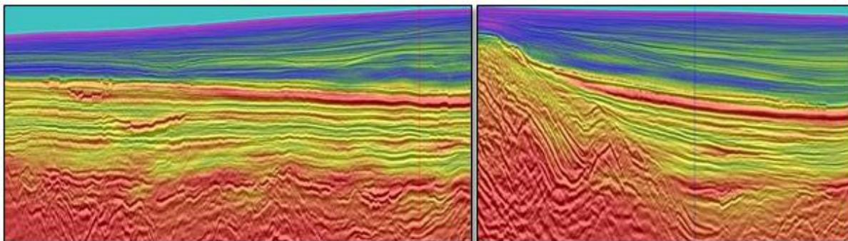
**Figure 1** Crossline (left) and inline (right) velocity model overlay after four passes of tomography.
