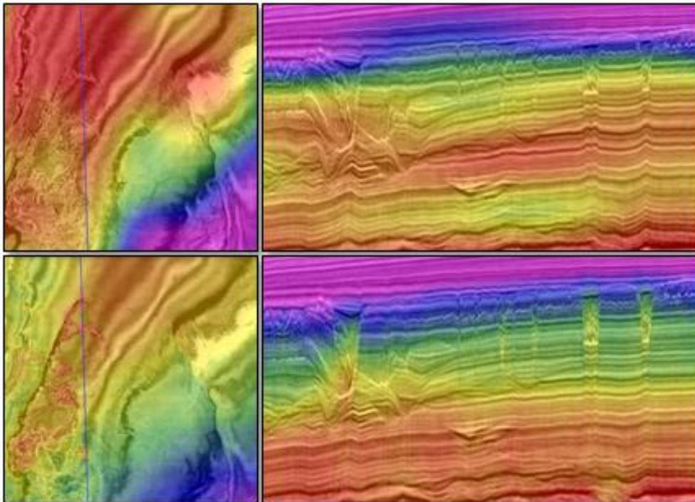
**Figure 2** Velocity model – depth slice and crossline section before and after FWI.
