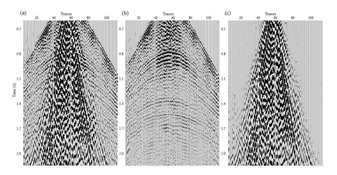
Figure 4: (a) A land seismic shot gather example containing strong ground roll. (b) Output data after suppressing ground roll using the proposed method. (c) Difference between the original data and output data.
