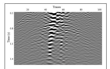
Figure 1: Example showing overlaped ground roll residue with reflection signal. In this example, the noise residue has similar dipping angle with the reflection signal at near offset. The downsclaed reflection mask cannot filtered out this kind of residue noise.
