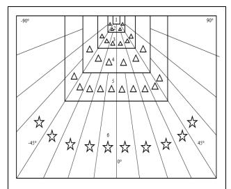
Figure 2: An example of curvlet coefficient panels used for ground roll suppression. Number 1 to 6 indicate the scales from low frequency to high frequency. The angle indicate the dipping angles for different scales. Stars represent the ground roll free panels used to calculate the reflection signal mask function, while the triangles mark the panels used to calculate the ground roll mask function.
