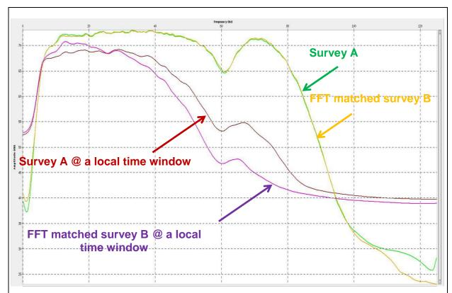
Figure 3: Spectra of survey A and survey B after spectrum matching applied by conventional FFT method. The spectra in green and yellow colors are from global window.
