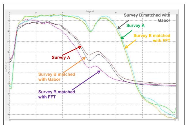
Figure 4: Comparison of spectra at both global and local time windows from survey A and survey B with application of different methods for spectrum matching.
