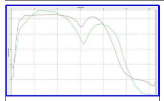
**Figure 2:** Spectra of surveys A and B to be merged. Significant differences in the spectra suggest the necessity of spectrum matching between the two surveys.
