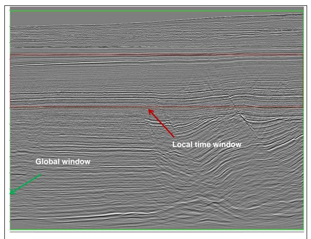
**Figure 1:** Example of seismic section used in the survey merge being discussed. The Global and Local time windows shown here are the spectral analysis windows used in the discussion.
