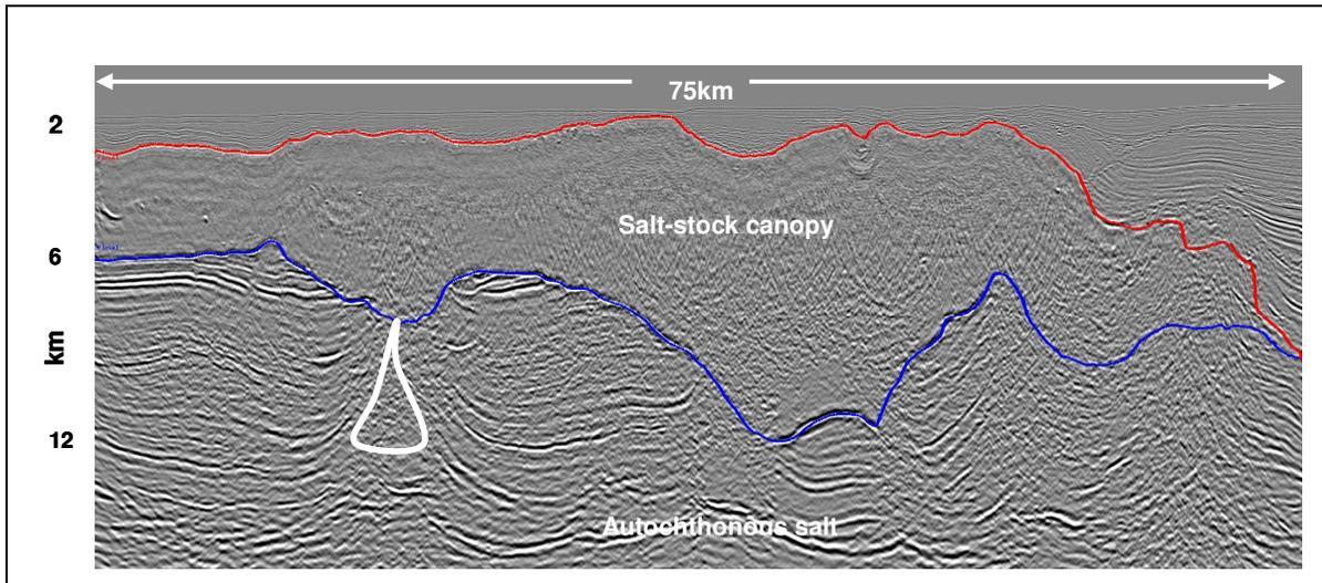
Figure 2: A north (left)-south (right) seismic section in deep water Walker Ridge area (water depth > 2km) shows a massive salt-stock canopy overlaid by thin suspension sediments. Opposite dipping events below the base of salt suggests a possible salt feeder/stock (highlighted in white).
